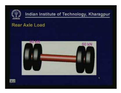
These axles can be of different configuration. They can have single wheel on either end or they can have what is known as dual wheel set.
