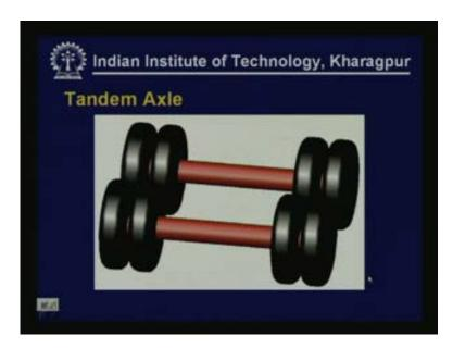
Besides the axles that have single wheel on either side dual wheels on either side, we can also have what is known as a tandem axle as shown above. Tandem axle is nothing but two separate dual wheel axles but working as one single unit. There will be a mechanism to ensure that the load transport is there on both the axles and both these axles together will function as one single unit called as tandem axle.
