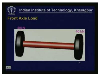
For example, let us assume the front axle of this particular vehicle had one wheel on either side. Then as indicated there it was carrying 80 kilo Newton. So if you assume the load to be equally or uniformly distributed over the entire vehicle from left to right, then we can assume the load to be distributed equally on both wheels and it should be about 40 kilo Newton each.
