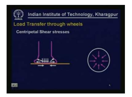
We can also have centripetal stresses on the pavement surface acting within the contact area. These occur because of the inflation pressure acting in different directions and then trying to push the tyre away. As a result we have this centripetal shear stress acting within the contact area.
