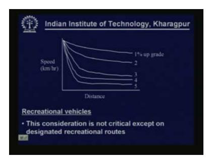
Here it is shown that, at various longitudinal grades, how the speed is reduced over distance. It is clearly observed that more the grade, more is the reduction in speed and also the speed generally reduces more as the distance is more.
