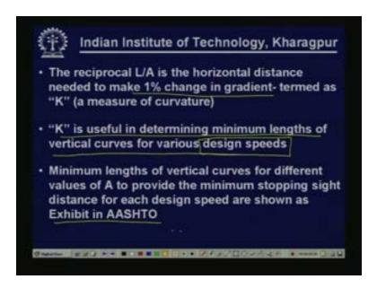
Now the reciprocal of this is L by A, which is nothing but the horizontal distance needed to make 1% change in gradient. That means what is the horizontal distance required to make a 1% change in grade. That means per percent change in grade what is the length of the curve that is required? This is termed as K factor and we call it as K. It is nothing but a measure of curvature. K is useful in determining minimum length of vertical curves for various design speed.
