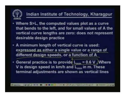
Now, again where S > L that is left side of this dotted lines which represent S=L, the computed values plot as a curve that bends to the left and for small values of A the vertical curve lengths are 0.
