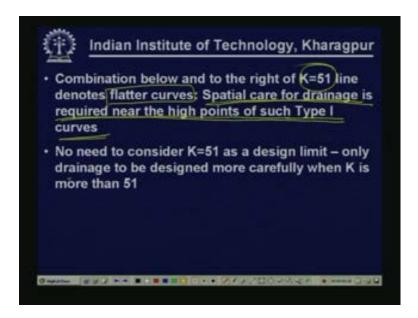
Of course, if it is more than 51, then special care should be taken for drainage near the high points of such 'Type I' curves. If K is more than 51 that means they are essentially flatter curves. Therefore special care is necessary for drainage near the high point of such 'Type I' curve. However this K equal to 51 should not be used as a design limit.
