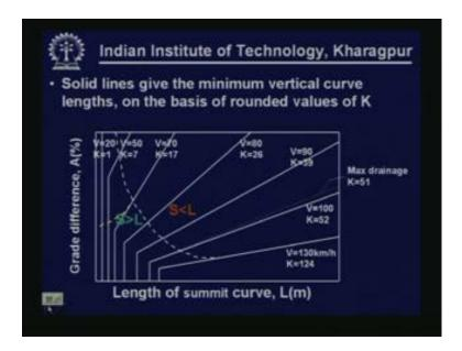
Look at this graphs or exhibit. The solid lines shown in white colour in the graph are the minimum vertical curve lengths on the basis of rounded values of K. Note that it is based on the 'rounded values of K'.
