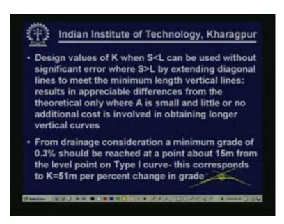
I have mentioned it once again, design values of K when S < L can be used without significant error where S > L by extending diagonal lines to meet the minimum length vertical lines; and this results in appreciable difference from the theoretical calculation only when A is small. If we draw the theoretical curve that takes a turn towards a left and that gives value even 0. So these vertical terminal adjustments are made.
