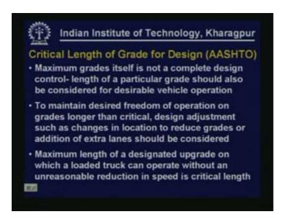
Coming to the critical length of grade for design, we have talked about the maximum grade but maximum grade itself is not a complete design control. Length of a particular grade should also be considered for desirable vehicle operation. This is purely based on the fact that, if the length is more and as the grade is also more, then there is a reduction in speed. We have already seen this trend earlier.
