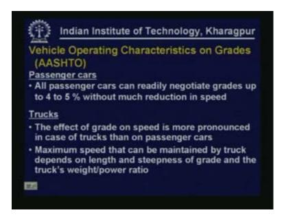
It is observed that almost all passenger cars can readily negotiate grades up to 4 to 5 % without much reduction in speed. That means if the grade is up to 4 or 5 %, then it is generally acceptable to cars, they do not face many problems. Now, what happens if the design vehicle is a commercial vehicle or a truck instead of a car?
