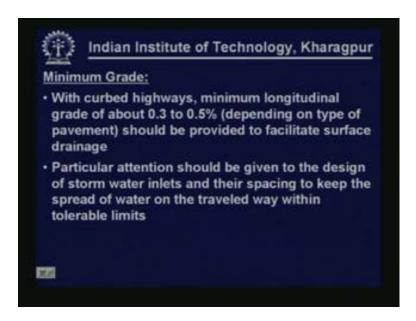
Let us look at the other extreme that is the minimum grade. With curbed highways minimum longitudinal grade of about 0.3 to 0.5% should be provided to facilitate surface drainage. Obviously what should be the exact grade between 0.3 to 0.5%? That will depend on the type of pavement.
