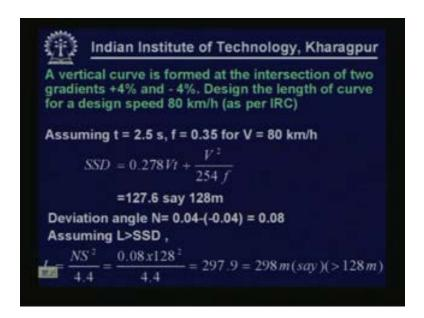
Now a vertical curve is formed at the intersection of two grades 4% and -4%. So this is clearly a case of a summit curve. One can calculate what the required stopping sight distance is, and then the deviation is the algebraic difference which is 0.08. Let us assume L is greater than SSD accordingly NS square by 4.4, we calculate the length it is 298 which is greater than 128. So our assumption is correct. Hence in that way we can calculate also the length of curve.
