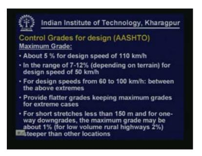
So, based on the vehicle operating characteristics, the control grades for design are recommended. There are two types of limit, one is the maximum value and the other one is the minimum value.
