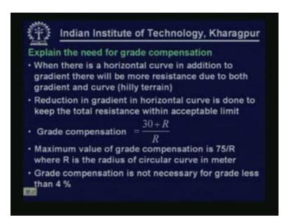
Why the grade compensation is required? If horizontal curve is there and vertical curve is there, the component of tractive effort available in the direction of movement becomes lesser. If it is 't', the tractive effort and if it is a horizontal curve only the 't cos alpha' component is available. So even if the grade is there, it is further a component. Therefore a kind of grade compensation is required for smooth operation of vehicles.
