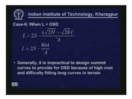
For L < OSD, again the same basic equation, only thing capital H or small h are same here. So accordingly values are to be provided. But generally it is found that if the length is to be designed to provide adequate overtaking sight distance the length requirement is much
