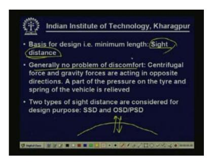
Let us take this one, so this is the curve. So when vehicle is negotiating this curve the centrifugal force is acting in the upward direction and the gravity force is acting in the downward direction
