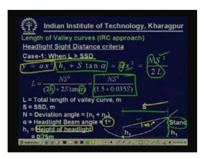
Let us see the length of valley curve considering the Headlight Sight Distance criteria. In this case critical position of vehicle is at the bottom of the curve at the lowest point on the curve. Say this is the point the lowest point on the curve let us again consider case one where L is greater than SSD. In this case it is lowest position on the curve that is the critical position and again the equation we can consider as Y equal to ax square.
