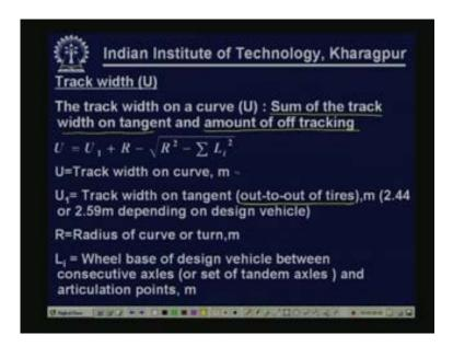
So it can be expressed by simple equation like this;  $U = U_1 + R$  – root over R square – sum of  $L_i$  square where U is the track width on curve,  $U_1$  is track width on tangent as per AASHTO procedure it is 2.44 or 2.59m depending on the design vehicle, R is the radius of curve or turn in meter and  $L_i$  is the wheel base of design vehicles between consecutive axles and articulation points this is also expressed in meter.
