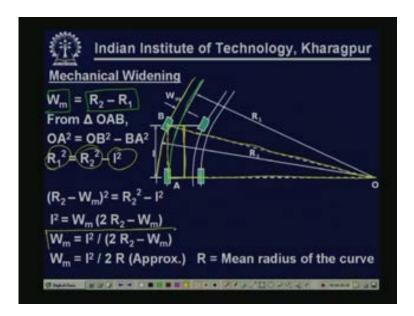
So obviously if  $R_1$  is the radius of curve considering the path traced by the outer rear wheels and  $R_2$  is the radius of the curve considering the path traced by the outer front wheel then the requirement of extra widening Wm is nothing but the difference between the two  $R_2 - R_1$ . Now if we consider this triangle OAB may be again shown by the yellow line OAB so if we consider this triangle A is the position of the outer rear wheel, B is the position of the outer
