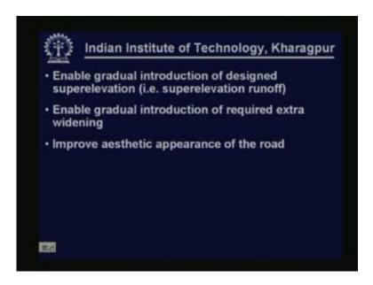
Enabling gradual introduction of design superelevation that is superelevation runoff particularly this length and also enable gradual introduction of required extra widening and finally it improves the aesthetic appearance of the roads. So those are all the advantages of using transition curve.
