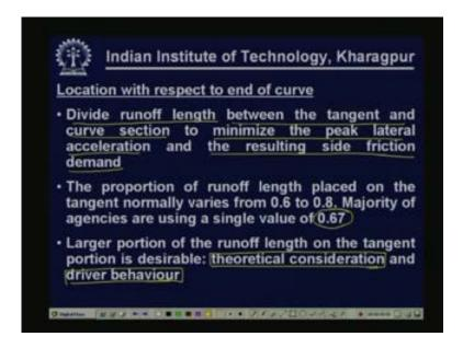
Larger portion of the runoff length on the tangent portion is desirable from theoretical consideration and also from the consideration of driver behavior.
