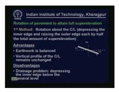
Now we have got uniform slope equal to camber. Now that slope is to be further rotated to have the required amount of superelevation. Again there are two possible alternative methods. In method 1 rather there are three different methods.
