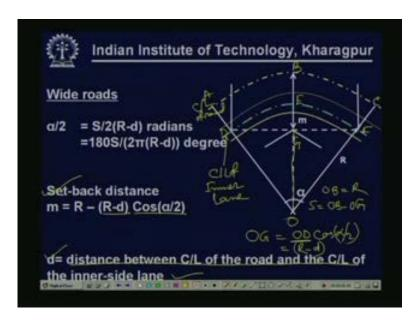
Suppose we consider a wider road, now in case of a wider road vehicle is placed towards the center line of the inner length. Now this is the center line of road and this green line indicates center line of inner length. So in this case set-back distance is from point this is A, this is B, this is C, this is D, say E, F, G and this is O. So principally or conceptually it is the same.
