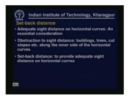
Now you know that at every point on highway adequate sight distance should be available. We have discussed about various types of sight distance. The minimum requirement is the Stopping Sight Distance or the SSD. The horizontal curve is a location where there could be problems of sight distance. So adequate sight distance must be ensured at all horizontal curves for safe and efficient movement of traffic and sight distance at horizontal curve is an essential consideration.
