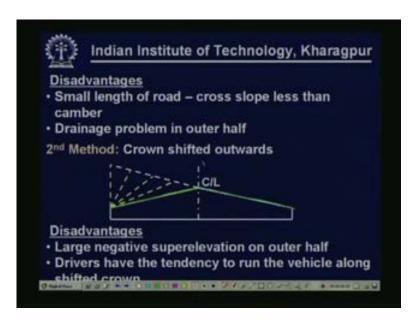
So if you see now the disadvantage basically is, small length of road will have cross slope less than the camber. Therefore there could be drainage problem in the outer half and one may find that outer edge or that portion may get damaged much early. Therefore, in order to overcome the problem associated with the first method the second method is sometimes adopted.
