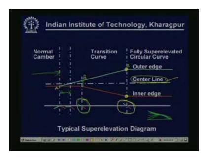
This is the normal cambered section, this portion up to this is the normal cambered section so you have level for the outer edge and the inner edge they are same, that is shown here by the red line, in fact the red and green line are going together. (Refer Slide Time: 25:45). Now this point onwards we are rotating the outer edge.
