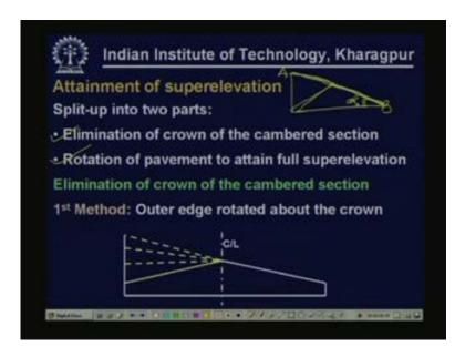
This can be split into two parts; one is elimination of crown of the cambered section that is part A. That means the original cambered section say it is like this. Elimination of crown means we have uniform clause cross slope equal to the camber. That means earlier the section was like this. After this part or after this stage we expect a section with uniform cross slope equal to the superelevation.
