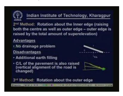
So may be in earlier case after the first stage it was like this. Now we don't change this inner edge, we now rotate the pavement further to have a cross slope like this. So what is happening is the pavement is rotated with respect to the inner edge. Now inner edge level is not changed so a major advantage with this method is there is no drainage problem now because we have not changed the level for the inner edge, it practically remains unchanged. However, this method has its own disadvantages.
