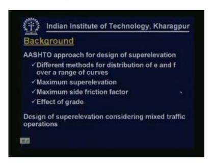
In the last lesson we discussed about the AASHTO approach for design of superelevation. In particular we talked about different methods for distribution of e and f over a range of curves. We also discussed about maximum superelevation rates which are described by AASHTO under different conditions. We talked about maximum side friction factors depending on the speed level and also discussed about the effect of grade on superelevation design.
