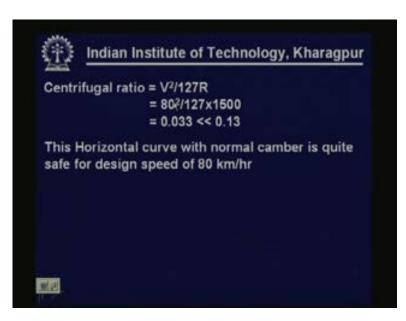
The centrifugal ratio V square/127R we calculate it as 0.033 so it is certainly lesser than 0.013 so again the normal camber section can be written and still the design will be safe in this condition.
