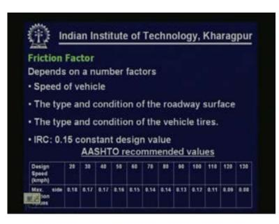
Since we are talking about the coefficient of friction what should be the design value. Actually the friction factor or the coefficient of friction depends on a number of factors. For example, speed of vehicle, the type and condition of the roadway surface, type and condition of the vehicle tires etc.
