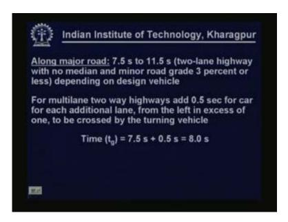
Along the major road normally it is 7.5 seconds to 11.5 seconds that is for car. But for multilane highway 0.5 seconds for each additional lane is to be added that is to be crossed by the turning vehicle. Since it is a full length road so one additional lane is to be crossed. Instead of one lane it is to be two lanes so 0.5 second is added making it 0.8 seconds and that's the effect of width.
