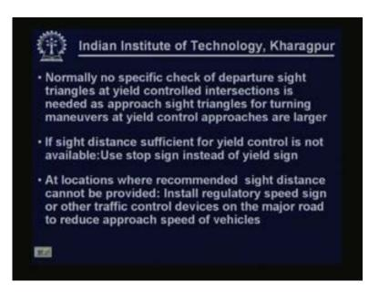
Normally no specific check for departure sight triangles at yield controlled intersections is needed as approach sight triangles for turning maneuvers at yield control approaches are larger. So if we design sight distance considering yield control approach and considering the left turn and right turn without stopping then the required sight distance whatever will be obtained will normally be larger than the stop controlled requirement. So no specific check is normally required.
