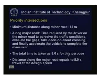
For priority intersections we have to find out the minimum distance along the major road and the distance along the minor road to get the required sight triangle.
