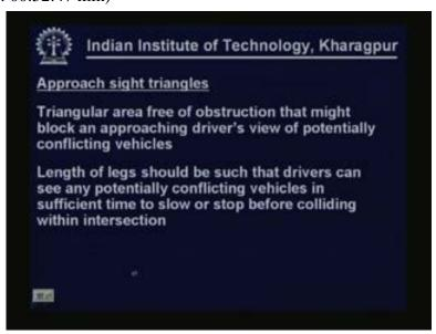
The approach sight triangle is the triangular area free of obstruction that might block an approaching driver's view. That means vehicle is in motion of potentially conflicting vehicles.
