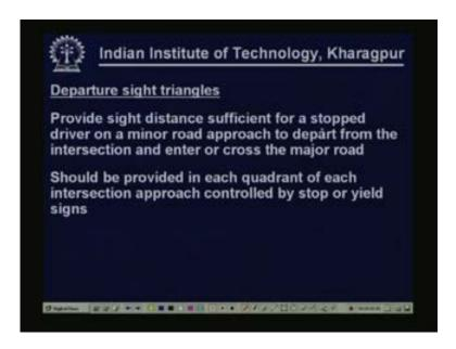
For departure sight triangles it is the same sight triangle same concept but here it is to provide sight distance sufficient for a stopped driver on a minor road approach to depart from the intersection and enter or cross the major road. So one case approach sight triangle is for moving vehicles, departure sight triangles is for stopped vehicles.
