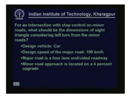
The last question was for an intersection with stop control on minor roads what should be the dimension of sight triangle considering left turn from minor road?
