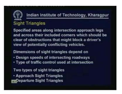
Let us now try to understand the concept of sight triangle. Sight triangle is specified areas along intersection approach legs and across their included corners which should be clear of obstructions that might block a driver's view of potentially conflicting vehicles. That means when vehicle is approaching an intersection it is basically that triangular area near the corner which should be free from all kinds of obstructions that might block the view or the sight the line of sight.
