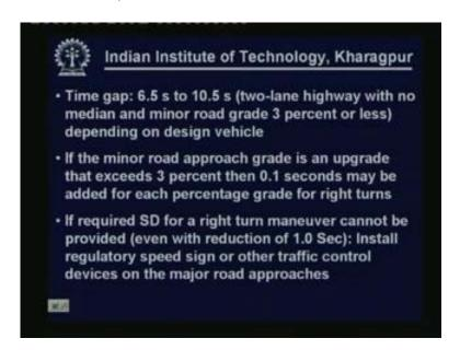
It is observed that vehicles normally accept for right turn, vehicle accepts a slightly lesser time gap; AASHTO says that one can consider one second lesser time as compared to what is recommended for left turn. So for left turn it was 7.5 to 11.5 here it is 6.5 seconds to 10.5
