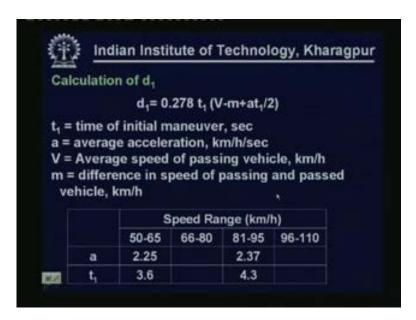
Now d 1 can be calculated with the help of this formulation 0.278 t 1 into V minus m plus a t 1 by 2. We have discussed the basis for this equation. Now, for different speed ranges the values of a that is the average acceleration and the value of t that is the time for initial maneuver they are decided so depending on the speed range the values can be selected from manual.
