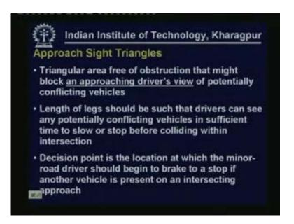
Approach sight triangle as given here is the triangular area free of obstruction that might block an approaching driver's view of potentially conflicting vehicles. I would like to draw your attention on this particular aspect and approaching driver's view. That means when a vehicle is approaching the vehicle is in motion so at that time what is the triangular area that should be free from obstruction for the approaching vehicle.
