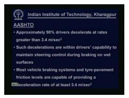
Coming to the AASHTO it is found that approximately 90 percent drivers they decelerate at rates greater than 3.4 m per second square. Also, it is found that such decelerations are within drivers' capability to maintain steering control during braking on wet surfaces because wet surface is
