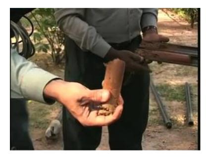
And you can see that the sample was moist near the top and it was becoming dry as we went downward. So, this has got a lot of sand and silt and other fine grain soils. It has got some cohesion as well and that is how we identify the sample and this is the sample which is near the bottom end of the sample.
