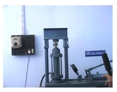
The sample is in between two points. You just observe the sample. It is going to crack once the point load reaches the failure value; the sample failed and the reading was roughly about 14; 14 kg per square kg per square centimeter at which the sample failed.
