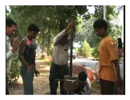
So, you see that the first 150 millimeter penetration is completed with only one blow; the soil is quit soft here. Then we are going to go with the next penetration of 150 millimeter.
