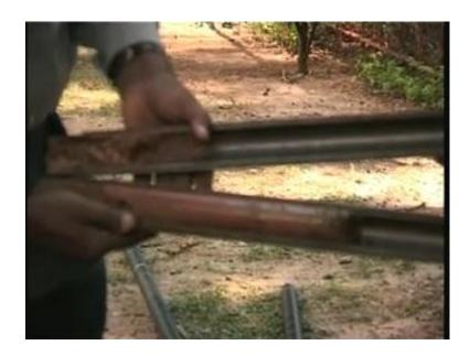
This particular sample is visually identified in the field and it is also saved. Some of the samples is also going to be saved for moisture content determination. So, if you recall this is the bottom end of the sample and that is the top end of the sample.
