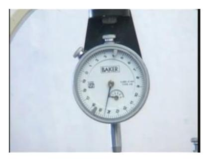
You can see that the loading range here is gradually decreasing. In other words, it is taking more and more movement to mobilize a certain amount of soil reaction. It is virtually stand still; it is not increasing any more. So, we are going to terminate the test here and you can see the deformed pattern from the bulging out as I was mentioning before of the sample.
