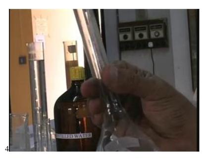
In fact, this particular flask is calibrated to be of 250 milliliter of volume at 27 degree Celsius and you can see that there is a mark on the stem of this particular flask and we are going to take distilled water exactly up to that mark. We are going to find out what is the weight of the flask plus distilled water and then we are going to take the distilled
