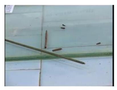
And you see here that the sample has been dried up and it started to crack. The thread has started to crack as soon as it has reached about 3 millimeter diameter and the cracks are
