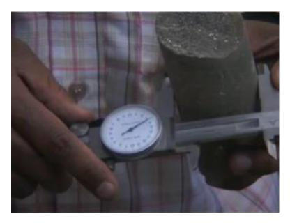
So, the sample diameter in this particular case is 53.36. I want to take a few more readings. So, here I am getting a value in this direction. In other orthogonal direction, I am getting a value, different value. Here it is 53.26. So, by taking such measurement in at least four orthogonal directions, whatever average diameter you get, you need to use that average diameter in your point load index calculation.
