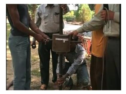
This is a hammer called donut hammer. This hammer has got a weight of 65kg. It is going to fall through 750 millimeters onto the hand wheel here which is underneath the hammer, which may not be visible from where the camera is.
