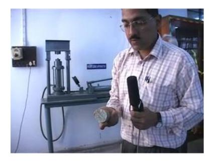
So, this is the face where the sample broke and we are going to record the point load, actually the pressure which is 14.7 kg per square centimeter at which the sample failed. So, I am recording it here.
