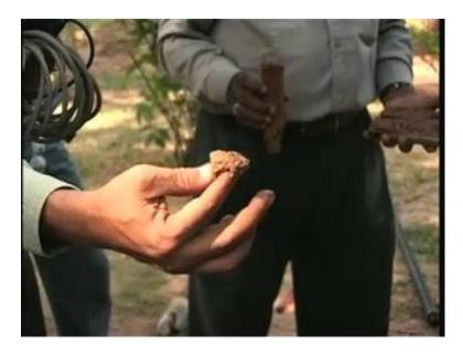
So, this sample is saved for grain size distribution and finding out the natural moisture content of the specimen. That is it.
