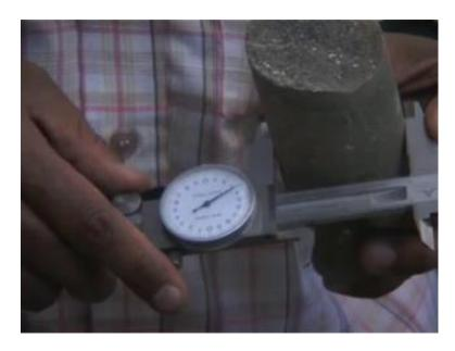
So, here again we are getting a readings of roughly 53.26 millimeter. all right. So, let us say, let us say the diameter of this sample is about 53.3 millimeter and we are going to use that 53.3 millimeter in our point load index calculation. So, this one, this sample here is 53.3.
