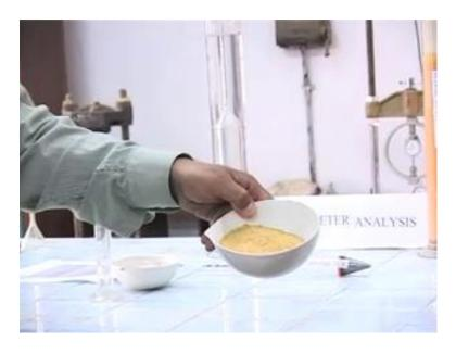
And what we are going to do with this particular sample is we are going to prepare a slurry of this particular soil sample, which has got, for which we want to find out the grain size distribution by taking 50 grams of the soil and making it mixing it up with water to make slurry of approximately one, exactly one liter. And we are going to place it, place the slurry making sure that soils are not readily settling in a sedimentation jar.
