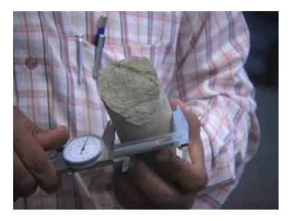
So, this sample, although it was obtained using the same reading, similar very similar reading, that similar reading equipment, the diameter is slightly larger than the one on my left hand and that is because of the durability of this sample. This, the sample that I am holding in my left hand is slightly more friable and slightly less durable than the one that I am holding on my right hand here. all right. Now, let us do the testing.
