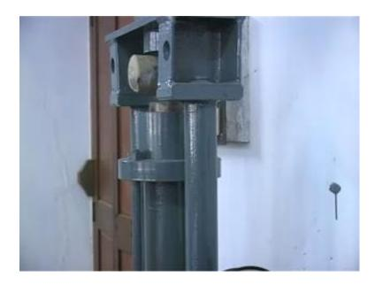
We have got the second sample and now we are trying to note the point load. You just look at the dial gauge reading. It is going to start mounting and when the sample fails, it is going to suddenly drop.
