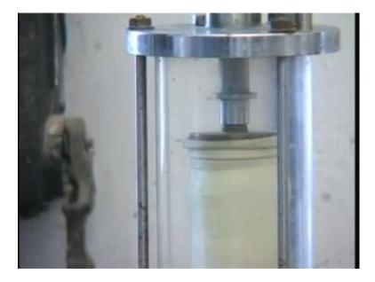
The way the data are analyzed is by calculating what is the axial stress the sample is being subjected to and plotting the axial stress versus the axial strength which is the changing length of the sample in the axial direction divided by the original length of the sample.
