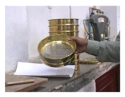
So, you see now after shaking of 10 minutes, we got the sieves back and as you recall that this was the coarsest sieve and in this one we do not have any coarse soil retained. (Refer Slide Time: 04:35)
