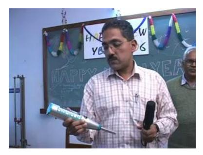
This is the instrument that we are going to use for nondestructive testing of a rock mass. It is very simple index really. So, what happens here is that we are going to push the instrument in and we have to make sure that this particular knob is stressed when the rebound occurs in order to measure the rebound value and the reading is going to appear on this particular scale here.
