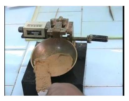
So, now, you see now we are preparing the pat in the pan making sure that there is no air entrapment within the volume of soil and the surface of this particular pat should be approximately horizontal. And then we use the grooving tool, as you see here, to cut a groove at the center of the pat, of the clay pat or pat of fine grained soil, and this is the groove that we construct, that we have constructed here using the standard grooving tool.
