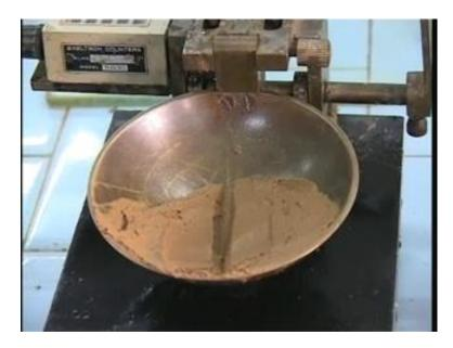
And you see here the pat is closed by an amount of approximately 12.5 millimeter and closure is approximately counted from there to about there and the number of blows in this case is much larger than 25. And what we are going to do? We have to keep on adding a little bit of water to the sample until we get the groove to close by 12.5 millimeter exactly on the 25th blow. And for doing that, what do we do?
