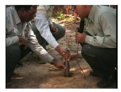
So, now, we have got the setup into the ground and what we have got here is a standard spt hammer mounted on the spt rod.
