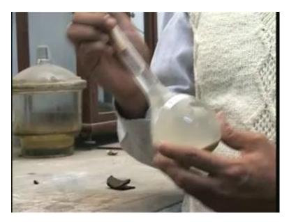
So, here you see that the soil is kept under a vacuum pump kept under vacuum here and that is being shaken by my colleague here, so that the water, so that the mixture does not have any intrusion of air because that might actually, as I was mentioning that might, introduce some error in the estimated specific gravity of solids..
