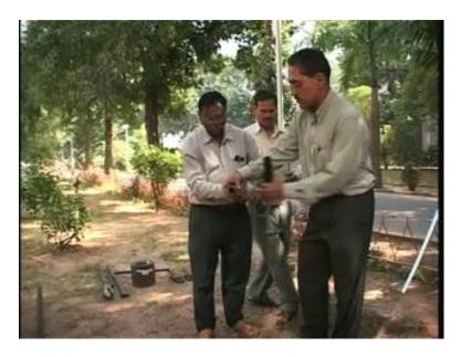
So, this is the cutting shoe which comes of like that and then the socket which connects the sampler to the spt rod. That also comes from the other side and then the portion in between splits into two different parts as you are going to see in the next little bit. You need a rod to do that and this is the two portions which split up like this one.
