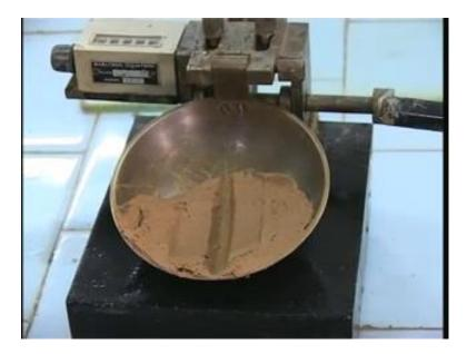
And then we are going to bounce it, bounce the pan up and down, bounce the pan up and down and count the number of blows that is required for the closure of the pat by an amount of 12.5 millimeter. You can see that the pat is gradually closing.
