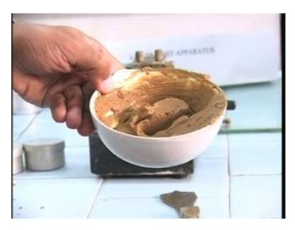
And what we are going to do? We are going to make a pat of this particular soil sample in this pan here.
