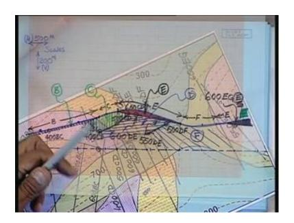
Now back to the other interfaces. Now we are going to get another one to the further right, and that is going to be between e and g. So, let us consider those strike lines. So, this is the strike line at 600 meter elevation between e and g and project this one up to 600. So, that is going to be the point where e and g is going to be separated. So, this is going to be 600 e g. And we have got another point further right that is going to be at 500
