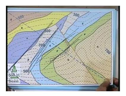
So, here again we have marked the strike lines, and again, you have to actually label the strike lines and project the strike lines up the appropriate values to demarcate the interfaces between units c and d in this case.
