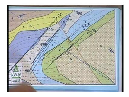
Because the strike lines that are bunching here they represent the interface between units c and d, and the strike lines that bunch out here they represent the interfaces between
