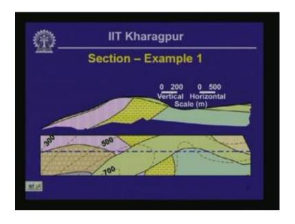
So, now I am going to also show you the result that we are going to get. So, this is the first example that we are going to consider. And here I have rotated the map, in fact, so that the section becomes horizontal actually on this particular slide, and the geologic section that is going to be prepared from this particular drawing is shown up above of the geologic map.
