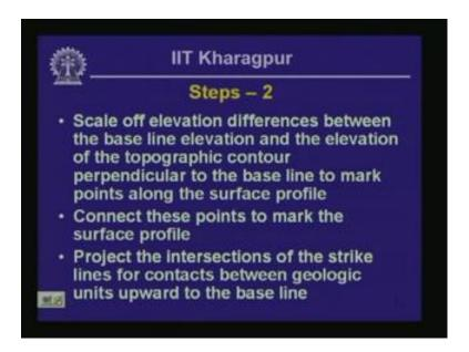
Then we are going to scale off the elevation differences between the base line elevation and the elevation of the topographic contour perpendicular to the base line to mark the points along the surface profile, connect these points to mark the surface profile. Then we are going to project the intersections of the strike lines which I illustrated a little bit before for contacts between all pairs of geologic units possible upward to the base line.
