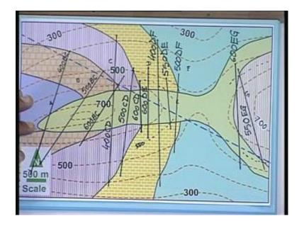
So, for example, the strike line on the left here which I am going to label, it connects the interface between b and c at elevation 400. So, let us label this one as 400 b c, then you can tell what is the next one. The next one actually connects again the interface between
