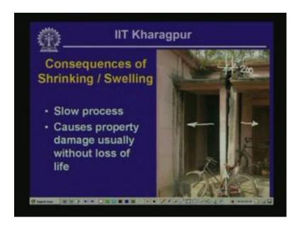
Now this is an example of consequences of shrinking and swelling; typically, the process is quite slow in many situations, because it requires entry and exit of water into the matrix of fine grained clay particles. So, the process generally occurs at a slow pace, and this, in fact, could lead to a severe damage of property, but usually the possibility of loss of life could be discounted. Now on the right, I show a picture of an office complex in
