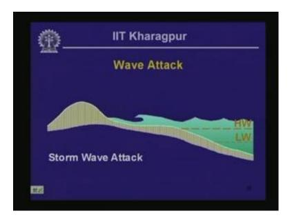
Then during storm wave attack, it is going to elevate the water height, and erosion is going to be caused by that, and the configuration is going to become like this.
