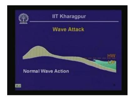
Normal wave action is then going to give rise to this type of configuration of the seafloor of the topography.
