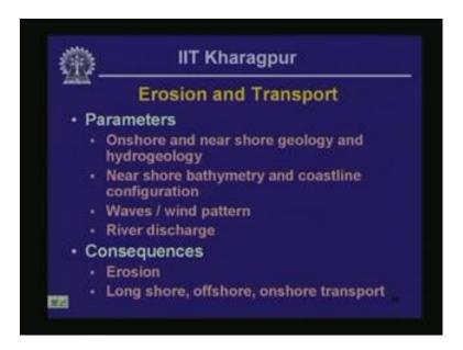
Erosion and transport is the consequence of these shoreline processes. One of the major consequences of these shoreline processes is erosion and transport. This is over and above the loss of life and property that is caused by the action of the waves themselves. And as engineering geologist, we are mostly linked with the mitigation of the hazards associated with erosion and transport due to all different shoreline processes that we listed a few minutes back.
