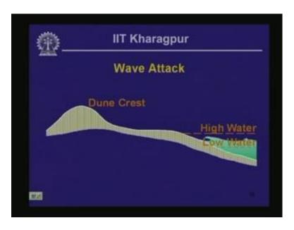
So, water level here is the normal sea water level in between low water and high tide level, low tide and high tide level. There is typically a flat lying area adjacent to the water line and that is the beach typical sea beach and on the landward end of the sea beach is often times we have got dunes that develop because of wave actions and deposition and transport.
