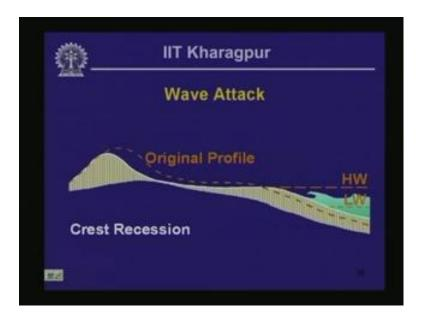
And if you superpose the original profile on top of the final profile, you can see because of the wave action, the dune crest has receded landward.
