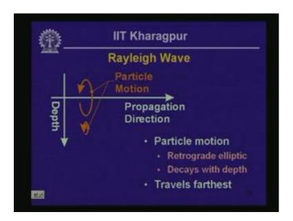
In Rayleigh wave, you have got retrograde particle motion taking place in an elliptical manner like that, and the extent of motion actually the intensity of motion decays as you go down deeper from the surface of the earth. So, here you have got a particle motion retrograde elliptic particle motion that decays with depth, and this particular wave actually travels the farthest. It does not decay as readily as P wave or S wave.
