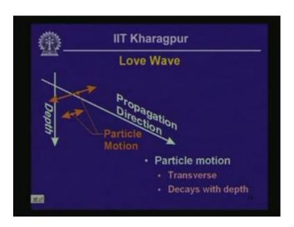
Love wave is very similar to Rayleigh wave except here the particle motion is transverse to the propagation direction, but here also the particle motion decays with depth.
