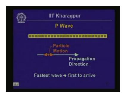
Now p-waves how they are developed, how they are generated is indicated on this particular animation. Here we actually hit a series of elements in that manner in the manner shown by the arrow there. Then what is going to happen? A deformation wave is going to propagate in that manner; here the propagation direction is like that, and the particle motion is parallel to the propagation direction. It is the fastest wave. So, that is the first to arrive from the focus to a particular site.
