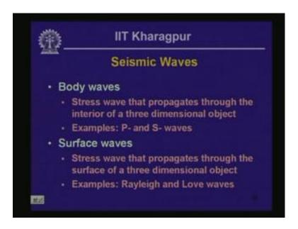
Now let us look at the features the characteristics of seismic waves. There are two types of seismic waves really. The waves it is exactly similar to, say, for example, if you throw a pebble on the surface of water in a pond or a water body. Then what you see is a wave is going to be triggered when the pebble hits the water surface. And the disturbance actually propagates radially from the location where the disturbance was originally
