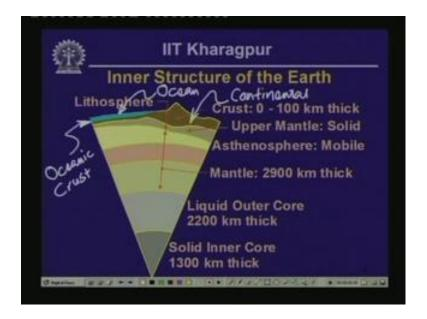
And here in this particular sketch I have shown the oceanic crust is on the left, and continental crust is towards the right. So, this one here is the oceanic crust. And you can see that oceanic crust is relatively much thinner in comparison with continental crust. So, this part here is continental crust, and this is the ocean that I have shown on this sketch, okay. So, that is the structure of the earth.
