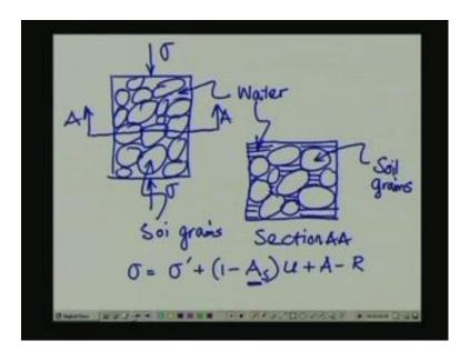
Let us say you have got an element of soil which is composed on several different grains, and what we have is a saturated sample and the pore space is full of water in this case. So, then we take a cut across the sample, and if you look at the plane view of this
