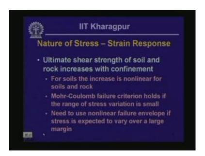
So, now what we are in a position actually to look at the major features of this stress strain response. What we have seen is that ultimate shear strength of soil and rock increases with the increase of mini normal stress or increase in confinement. That means, if you have got the same type of rock occurring at great depth underneath the ground surface as well as it has another at another level near the ground surface, you have got an
