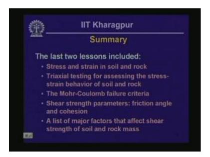
Summarize this particular lesson as well as the last one. We looked at the characteristics of stress strain behavior of soil and rock, looked at triaxial testing and how we can access the shear, how we can access shear stress strain behavior of soil and rock, then how we can obtain Mohr-Coulomb failure parameters associated with Mohr-Coulomb failure criteria from conducting triaxial tests, and we looked at a list of major factors that affect shear strength of soil and rock mass.
