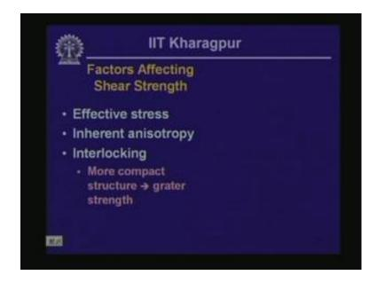
It is very important principle actually seminal. In fact, that leads to the entire development of this field of learning, then factors affecting shear strength. What are the factors that affect shear strength parameters? Number one is effective stress. So, higher the effective stress as we have noted that the shear express, the assembly can support is also going to increase.
