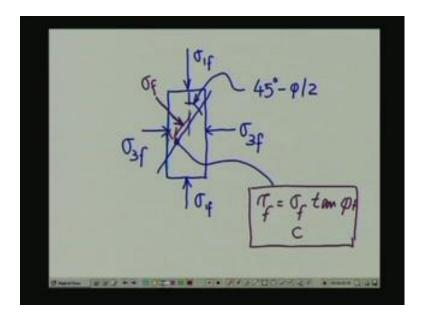
So, if you have got, if you recall that triaxial sample that we were testing sigma 1 f was in the vertical direction oriented in this manner, and sigma 3 f could have developed in
