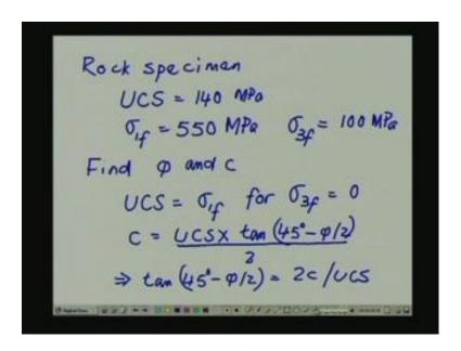
Let us consider a rock sample, rock specimen for which the UCS is equal to 140 MPa and sigma 1 at failure is 550 MPa in one triaxial test and sigma 3 at failure in the same triaxial test is 100 MPa. Now, our problem is to find phi and C for this particular rock specimen. So, how do we proceed?
