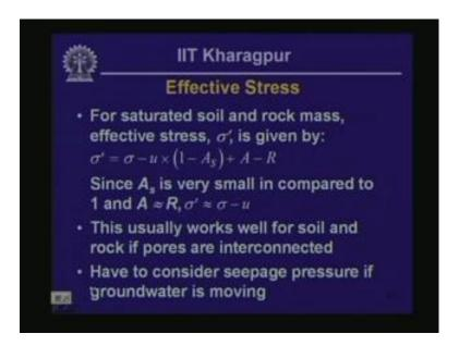
Now, we introduce the concept of effective stress for saturated soil and rock mass. Effective stress is given by this expression here, sigma prime equal to sigma minus u multiplied y 1 minus A S plus A minus R. Now, what are these trans is going to be let me explain that before I proceed any further.
