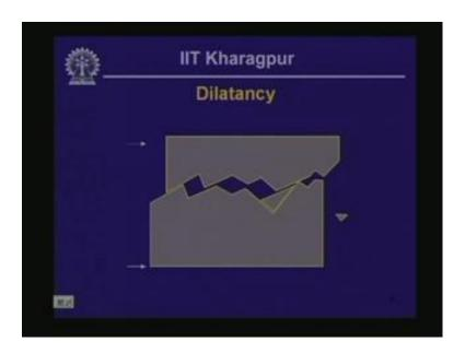
So, what happens here is that the top piece tries to climb up as it is shear to the right of this screen, and this include, this involves a change of volume and you should have also noticed that the void space in between the top space, top piece and the bottom piece increases and during this process and this type of behavior is called dilatancy.
