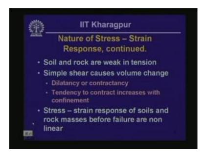
A few more features are soil and rock is weak in tension. They cannot take tension and that was clear from the failure envelope that we illustrated in the previous screen there.
