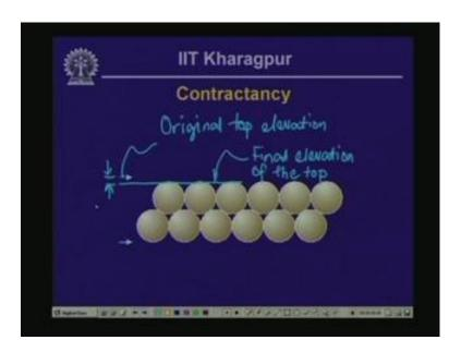
Let us consider the reverse of it and in this case, we are going to consider an assembly of spheres. We could have done the same thing using two pieces of rock which we were considering in the previous example, and going in the reverse direction in time, but in order to give you a new flavor I considered a piece of block of soil like material composed of uniform spheres.
