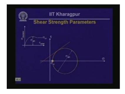
So, now we continue with the discussion that we started in the last time. If you recall, we were discussing how to analyze the data obtained from the series of triaxial tests performed on specimens of intact sample of rock or soil samples. Now, in the lesson that we had last time, we considered three different triaxial tests on three identical samples of rock or soil performed at three different shell pressures.
