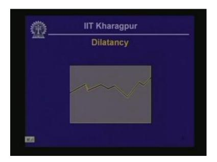
Now, we want to illustrate why there is a volume change when we apply shear stress on a soil or rock specimen. In order to illustrate that we consider a joint rock mass shown schematically on the screen there.
