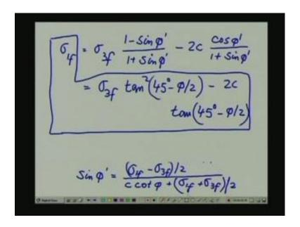
So, then what we do is we can collect tan and we can go through the geometry, go through the algebra, and we can show that sigma 1 f is equal to sigma 3 f multiplied by 1 minus sin of phi prime divided by 1 plus sin of phi prime minus 2 C cos phi prime divided by 1 plus sin of phi prime, and that in turn will give us sigma 3 f multiplied by tan square 45 degree minus phi by 2 minus 2 C tan of 45 degree minus phi by 2, and this is the relationship that we were trying to derive.
