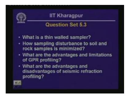
The questions are like this; the first one was what is a thin walled sampler? As I discussed in the previous lesson, thin walled sampler is a sampler which is basically a cylindrical tube with a wall, with a wall thickness of equal to or less than 10% of the sample cross sectional area. So, what is meant by that is say, we have got or here we are looking at the cross section of the sampler.
