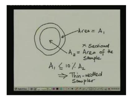
So let say, the outer diameter of the sampler is like this and the inner wall of the tube is like this; so this area, this is the cross sectional area, let say that is  $A_1$  and this area here is let say that is  $A_2$ ,  $A_2$  is the area of the sample, actually cross sectional area of the sample. So,  $A_1$  should be less than 10% of  $A_2$ ; then the sampler will be called a thin walled sampler. So, that is the definition of thin walled sampler.
