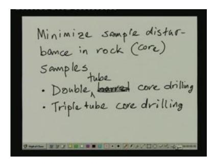
To minimize sample disturbance in rock samples, let say core samples of rock; so what we do we can either go with a double barrel core drilling or we could even go with a triple, actually a double tube, let us call it double tube core drilling, triple tube core drilling is even better. So, these are the possibilities and the procedures of, each one of these procedures were discussed in the previous day's lesson. So, these are the options that we have in order to minimize disturbance.
