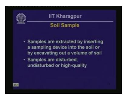
Now, soil samples are extracted basically, more usually they are extracted by inserting a sampling device into the soil or excavating out a volume of soil and we talked about some of these procedures of obtaining samples by excavating out a block in the previous lessons and also depending on what procedure is used during the sampling, the sampling could be disturbed or it could be undisturbed.
