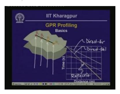
We have got a source of RADAR waves  $s_1$  and then we have got a detector called  $r_1$ . So, this is what we do basically; we use a source and we use a detector to find out what is the radar signature of the subsurface layers and in sense and then we alter the location, we take the source to a different location and we take the detector to a different location and by looking at signature for different detection signals or signals detected, we construct the profile of the subsurface layers.
