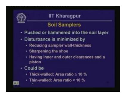
Now, what is a thick walled sampler and what is a thin walled sampler? Now, thick walled sampler are those samplers which has got an area ratio of greater than or equal to 10%, whereas thin walled sampler has got an area ratio of less than 10%. So, what is an area ration? Area ratio is the ratio of the area underneath the wall of the sampler to the cross sectional area of the soil sample that has been taken within the sampler during the sampling process. So, let me explain what I mean by that.
