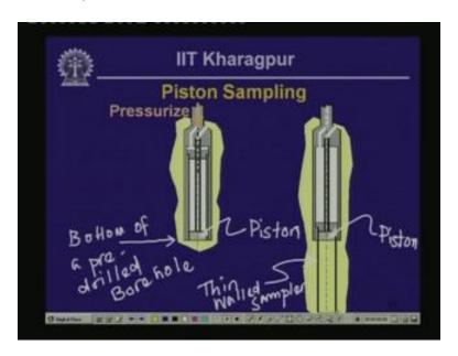
So, the sketch on your left actually shows the piston sampler placed at the bottom of the bore hole. So, this one here is placed at the bottom of the bore hole. So, this one is the bottom of the bore hole, bottom of a predrilled bore hole and then what happens is the piston is kept stationary - you can see that on the sketch to the right - piston is kept stationary and what is done is to insert the thin walled sampler into the soil underneath.
