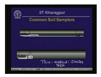
So, what is there actually like in the top sketch there, this particular picture also shows a partially cut view. So, the upper half of this picture actually it shows the outer appearance of this sampler and the bottom part shows the cut view or the section of the sampler. So, here obviously, this is your wall thickness; whereas in the previous in the thick walled sampler, you can see that that was the wall thickness. So, it is obvious that the wall thickness is quite small here.
