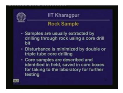
So here, the samples are extracted by drilling through rock layers, drilling through rock layers using a core drill. We have seen in the previous lessons, examples of core drill bit. Now, disturbance in this case is minimized by introducing a double or triple tube core drilling, core samples are described and identified in the field that are save in core boxes before taking to the laboratory for further testing.
