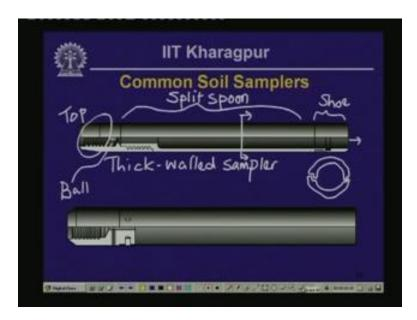
Then at the top end of the sampler also there is a threaded portion and this is the thread, you can see a threaded portion near the top end through which the split spoons are attached to an adopter and this adopter itself has got another set of threads, so these threads that I am talking about in this case; these threads, they screw on to the drilling rods such as aw rods or bw rods and also is of interest in this case that there is a ball, you can that there is a ball inside of the sampler.
