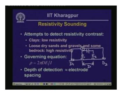
So, rho is the resistivity in this case, d is the distance between the electrodes that are used in order to circulate the current and these electrodes are placed at the ground surface where e is the voltage drop between the detectors and i is the current generated at the detectors.
