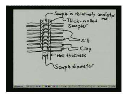
Let say, we try to introduce a thick walled sampler, cylindrical thick walled sampler into the ground, we are going to look at the definition of a thick walled sampler in the next little bit. Now, let say we are introducing a thick walled sampler like that. What is meant by thick walled sampler actually is that the proportion of the wall thickness, so this one is the wall thickness is quite large in comparison with the sample diameter.
