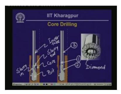
So, by introducing an inner tube we are not allowing the slurry that is getting flushed upward, this particular slurry to come in direct contact with the core that is taken within the sampling tube and because of the fact that there is no direct contact between the slurry and the sample that is getting into the tube, the sampling disturbance is going to be minimized, it is hoped.
