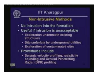
So, these procedures include seismic velocity profiling, resistivity sounding and ground penetrating radar profiling. We look at now the details of these things.
