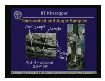
What you have got here? So, this one here is a sampler, this one and this one and this one here is the soil sample and you can probably if you can make out, if you look carefully, this particular sample is a sample containing, it is sand sample basically and it has got some gravel also in it.
