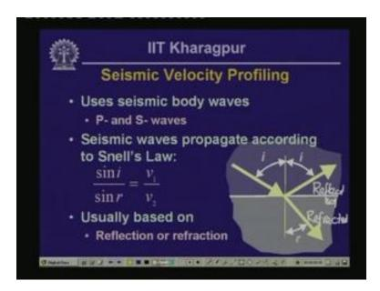
So, seismic velocity profiling use seismic body waves and the body waves are in a sense P waves or S waves. So, P waves are similar to the sound waves in a sense. In this case, the particle motion is in the same direction as the propagation direction. S waves on the other hand, the particle motion is in a direction transverse to the direction of propagation.
