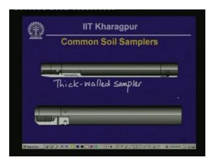
In this case, what we have is a shoe. So, this one here is the shoe and this one is the split spoon. Actually, this particular part has got two different or it is composed of two different segments. So, if we take a section there, then it is going to look like this. So, it is composed of two hemispherical segments; this is the cross section that I am trying to draw and then you can see that the bottom end, so this one enters the soil first, this end enters the soil first and this is the top end.
