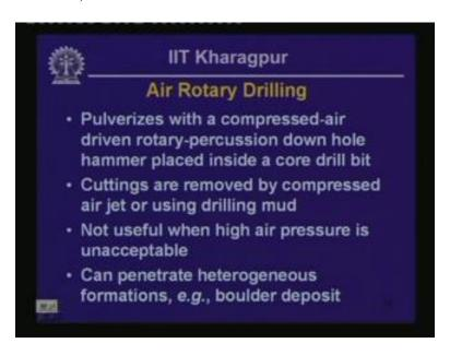
So here, we again pulverize the rock at the bottom of the bore hole and in this case, we use a compressed air driven rotary-percussion down hammer that is placed inside a core
