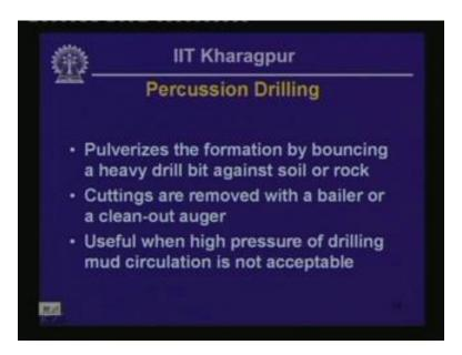
Percussion drilling typically also is a shallow drilling process, cannot proceed beyond say about 30 meters depth and this has got some of the advantages of the wash boring and the disadvantages that are associated with wash boring as well alright.
