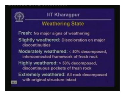
So, we begin with the description of weathering state. Now, a rock could be fresh if it is free from any aspect of weathering, relatively free from all signs of weathering. Then it
