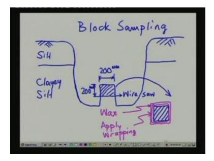
So, this is our pits and here, say we have got a shallow layer of slit near the surface underlained by a thick deposit of clayey slit. And, how the stratigraphy appears, that also becomes apparent from the description of the excavation process and identification of the samples from the site of the excavation like along these surfaces.
