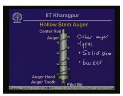
What you have got here is really, the hollow stem auger is the pipe that you see, this outer pipe is really the hollow stem auger and it has got auger head with the properly machined hard faced teeth that choose into the soils underneath and through the center of the hollow stem auger is another tube that runs through the center and this tube itself has got a pilot bit at the top of it and the chewing action is because of the rotation of the auger
