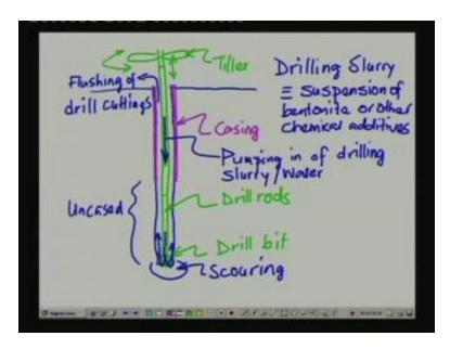
So, what is done here is to extend a relatively small diameter bore hole into the ground and the top portion of this bore hole is often supported using a metal pipe so that the soil after the bore hole is drilled, it does not collapse into the bore hole. So, this particular metal pipe is called the casing and then what you have got is a drill bit typically mounted at the bottom of a string of drill rods. So, these are drill rods and this one here is the drill bit.
