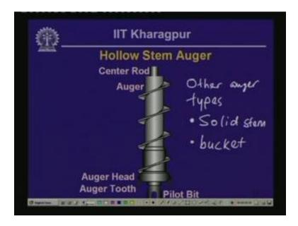
There are other types of augers also, other auger types as well which could be solid stem auger or a bucket auger. Bucket augers are of larger diameter typically, they can be upto 60 inches in diameter.
