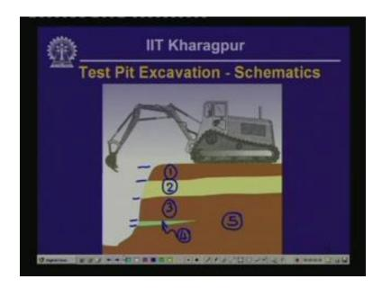
So, this one, this cartoon here shows a schematic of a test bit excavation process. Now here, what we see is that the test pit is actually proceeding from say soil number 1 near the surface, then it penetrated the soil number 2, all these things could be different types of soils like slit or sand or clay slit or any organic material whatever, then it enters soil 3 and then we have also got a lens really of another type of soil called the soil number 4 and we also have soil number 5 in this case.
