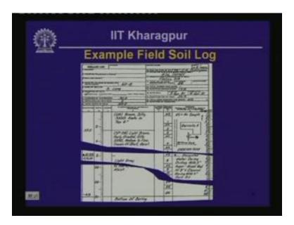
Now, this one here is an example of a soil log that is obtained during a drilling and here you can see that the top portion of this soil log, near the top portion of the soil log, we give the information regarding the location of the bore hole who is supervising the drilling, who is performing the drilling; then what kind of weather was there drilling work, when the drilling was done, what is the top elevation of the drilling and what was the procedure used in the drilling process.
