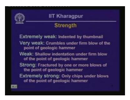
Then we have to describe roughly the strength of the rock specimen that is obtained during the investigation process. If the rock, again in the scale of increasing strength; we begin from the least strong specimen which is designated technically as extremely weak and this type of rock sample can be indented or can be marked with the thumbnail.
