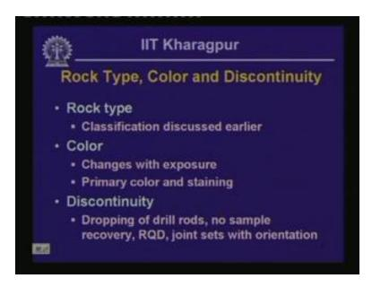
Then, we move on to rock type; color and discontinuity. So, we have to mention the geologic name of a given type of hand sample. Say for example, micaschist quartzite and this type of classification we have already discussed in detail when we were talking about different types of rocks.
