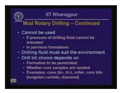
You also have to make sure that you use a drilling fluid which suits the environment which does not cause any damage to the environment and drill bit that varies quite a bit depending on the formation to be penetrated and whether core samples are to be obtained or not. Some of the examples are going to be seen in the next little bit, in the next sketch.
