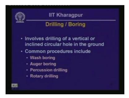
Now, first of all, we have to understand here is that the drilling process actually, the advantage, the relative advantage of drilling process as supposed to test pit excavation or trench excavation is that the drilling process can investigate a relatively thicker layer of soil and as it can extend to great depths; as we are going to see a little while later.
