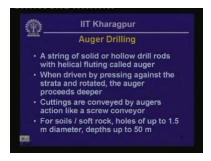
And, what is done is these augers they are kept pressed against the bottom of the stratum and they are rotated by mechanical means such as by using a hydraulic motor and as a result, the auger proceeds deeper and the soil cuttings that actually collect on the flutings of the screw like augers, they actually are conveyed to the surface, they get carried to the surface because augers also act as a screw conveyer.
