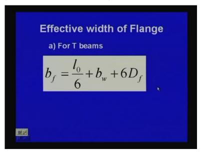
So, what is bf; bf equal to lesser of 1 by 6 plus bw plus 6 df, which comes as 5.5. Let us say e here divided by 6 plus 0.25 plus 6 times slab thickness 125 millimeter, which comes as 1.9166 meter. Let us take, 1.917 meter; b: centre to centre distance of beam and which equal to spacing that is 3 meter and we have to take out of this lesser of this 1; that which 1 is the minimum.
