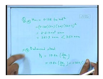
Mu1 what is Mu1 due to concrete failure Mu1 equal to 0.138 fck bd square Mu1 equal to 0.138 fck bd square due to concrete failure. It comes as 0.138 times 20 times 300 times
