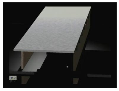
So, each of them will be t-beam and which has width of the web, depth of the flange, width of the flange and depth of the web also okay.
