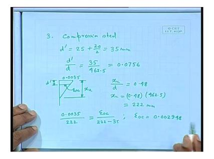
Number 3: compression steel d dash equal to 25 clear cover plus 20 by 2 35 millimeter. D dash by d 35 by 462.5 equals 0.0756. We can also write down as: this is d dash and the strain is 0.0035 xu, xu by d 0.48 xu equal to 0.48 times multiplied by d which is 462.5 which comes as 222 millimeter. What about epsilon sc then; epsilon sc will be this is
