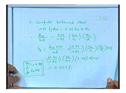
Number 2: compute balanced steel. Let us start from the beginning 0.87 fy Ast equal to 0.36 fck b xu. or Ast by bd equal to 0.36 by 0.87 fck by fy times xu by d; pt Ast times 100 divided by bd equal to I can simply write down 0.36 by 0.87 multiplied by fck by fy multiplied by xu by d times 100 times hundred equal to 0.36 by 0.87 times 20 by 415 times 0.48; xu by d equal to 0.48 for Fe 415 times 100 equals to 0.978 percent. So, balanced steel that is 0.957 percent.
