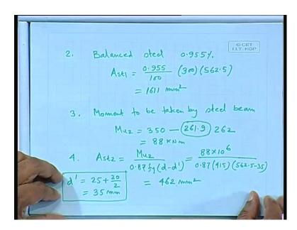
Number 2: balanced steel 0.955 percentage already we have computed. Therefore, Ast1 area of steel equal to 0.955 by 100 times 300 times the effective depth which comes as 1611 square millimeter. Moment to be taken by steel beam or in other way you have to provide the reinforcement now because, we are doing it to separate way 1 is that only isolated case of single reinforce section.
