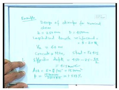
What about the shear force number 2: the that tow v equal to vu by bd v u equal to 60 into 10 to the power of 3 divided by 250 times 415 this 415 is effective with depth please note that the 1 the steel 0.578 Newton per square millimeter tow c max from table 20 of is 456; 2000, which comes as 2.8 Newton per square millimeter less than tow c max. From table 19, we shall get 100 ast by bd and tow c that we shall get 1.5 we are getting 0.72 this is in Newton per square millimeter, 1.75, 0.75.
