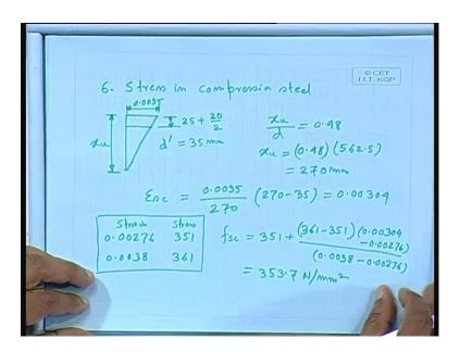
So, number 6: stress in compression steel. So, xu 0.0035 we are assuming, we shall provide 20 millimeter dia bar. So, clear cover 25 plus diameter twenty millimeter diameter equals 35 millimeter this is your the d dash; xu by d 0.48 xu equal to 0.48 times 562 .5 270 millimeter. Epsilon sc equal to 0.0035, which will be always less than this 0.0035 minus 35 equal to 0.00340.
