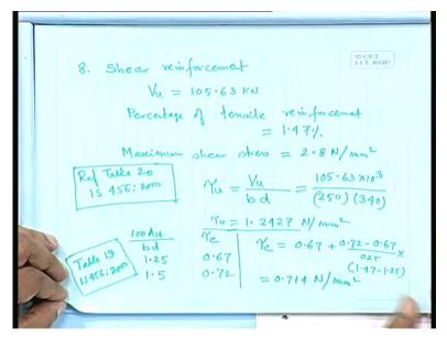
So, in our case; we can write down that tow v greater than tow c, but and tow v less than tow c max. So, no need of changing the ah your say section, but we have to provide shear reinforcement. So, shear the concrete due to concrete say and let us say, that 1 vc so, vc equal to 0.714 times, 250 times, 340, which comes as 60.69 kilo Newton. Shear to be
