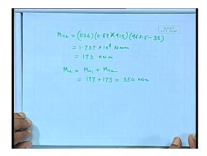
We can write down then Mu2; Mu2 will be equal to 1126 times 0.87 into 415 multiplied by 462.5 minus 35 which comes as 1.7378 equal to 100 say 73 kilo newton meter. Mu we can write down as Mu1 plus Mu2 equal 177 plus equal 173 equals to 350 kilo newton meter.
