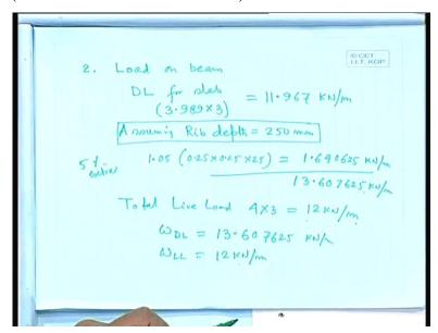
Now, we shall take that load on beam, individual beam that means; if we go back.
