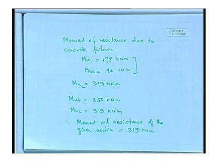
So, we have got 142 kilo newton meter Mu1 how much moment of resistance moment of resistance due to concrete failure Mu1 equal to 177 kilo newton because this is a balanced section and Mu2 we have computed 142. Mu 319 the sum of 2 this 2 sum of these 2 177 plus 1042, which comes as 319 kilo newton meter 1 we have got, we have got 2 values. So, we have got 2 values 177 plus 173 350. So, we can write down as say mut equal to 350 kilo newton meter.
