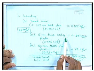
So, next 1 load on beam. So, we are getting this 1 that kilo Newton per square meter that is on the slab.
