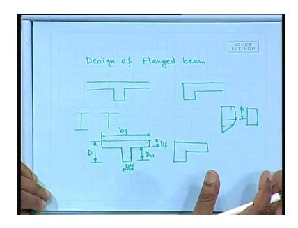
We shall do in the next class, since we have time little bit, we shall do the design of flanged section, flanged beam as I have mentioned, this is your slab and beam that the support at the end it generally comes we can call it as inverted L. We take whenever, it bends we take certain portion from both sides or from this side we take that is called flange, you can say that you say wave type of thing T beam like this.
