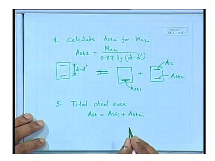
Number 4: Calculate Ast2 for Mu2 Ast2 equal to Mu2 divided by 0.87 fy and the lever arm d minus d dash for your reference again we are taking the section and d minus d dash. Ast2 means total area of steel that you are providing out of that you have 1 portion due to your balanced section. So, a section this section I can make it as let us say equal to this is equal I can consider, a section of same width and depth, but, having only tensile reinforcement here.
