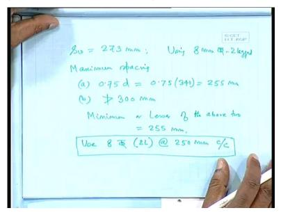
We shall provide the t-section, we are here 125. And this 1 250; we have 4 420 and the stirrup other 2 bar, we are ah just providing say: that we need not specify here, but anyway because for our design we shall not specify. So, we shall get 250, 420 tor 8 tor 2 legged at the rate of 250 millimeter centre to centre. Concrete m 20 steel fe 415; that only we have taking fe 415. So, anyway so, that we have used this 1; clear cover.
