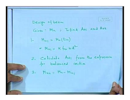
Let me continue, the part 2 of design of doubly reinforced beam. Let us check the procedure of design of beam. We have done the analysis, here given Mu and we have to find to find Asc and Ast area of steel in the composite side, area of steel in the tensile side. So, the steps find Mu1 equal to say Mu lim the limiting moment that balanced moment.
