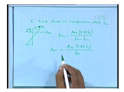
Number 6: find stress in compression steel. Let us say, that is fsc, we can find the fsc how shall we find out. This is at a distance d dash this is 0.0035. We can get the corresponding strain in the steel level epsilon sc, we can get the corresponding steel level in epsilon sc when we shall we get epsilon sc either from the carve either from the carve or from the table there where you have made it from there we can find out the corresponding stress fsc.
