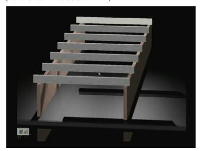
Covered by the roof slab. So, this is your different beams but, we have constructed these beams integrally with the slab. So, we can take action of the t-beam.
