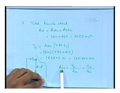
What about the total tensile steel; total tensile steel, Ast equal to Ast1 plus Ast2 1611 plus 462 equals 2073 square millimeter. We know 462; 462 is the area of steel. What is the corresponding force. Let us say, tensile force T2; tensile force T2 equal to Ast2 times 0.87 fy equal to 462 times 0.87 into 415. This is the force. So, 462 times 0.87 times 415 comes as 166805 newton equals 166.805 kilo newton this is the force.
