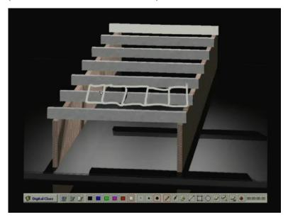
So, if we take this 1 you can get the load 3.898 kilo Newton per square meter for dead load and for live load 4 kilo Newton per square meter and which you are getting within this area within this area you are getting this load. So, now where to take the loading on the beam load on beam. So, how much is the load on beams. So, dead load for slab that we have already computed and that we are assuming and here we are assumed certain rib depth rib 250 millimeter.
