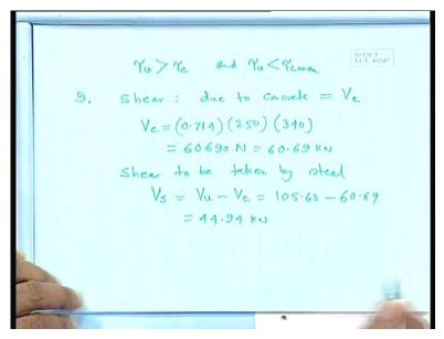
What about vus. Let us go the next page then vus that is: as per the code 0.87 fy times, asv times d divided by sv the spacing asv by sv equal to vus in our case divided by 0.87 fy d or asv by sv equal to 44.94 into 10 to the power of 3 divided by 0.87 415 times, 340 equals 0.366. This the 1 asv by sv we can get 0.366. If we use. Let us say, use eight mm tor. So, asv and we shall use 2 legged therefore, asv equal to 2 which will be equal to say 2 into 50 equal to say 100 square millimeter.
