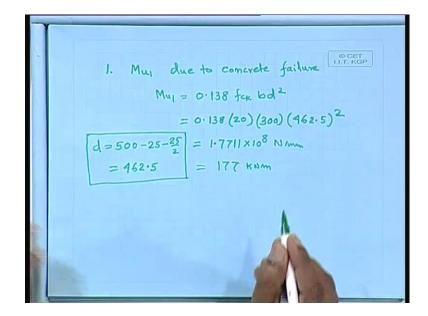
Number 1: Mu1 due to concrete failure. Mu1 equal to 0.138 fck bd square equal to 0.138 multiplied by 20 times 300 that is: the b what about d let us calculate d. D equal to capital D minus clear cover minus 25 by 2, which comes as 462.5 The top and bottom
