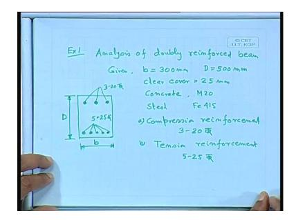
Example 1 analysis of doubly reinforced beam given b equal to 300 millimeter d 500 clear cover 25 millimeter concrete m 20 steel Fe 415 compression reinforcement 320 tor tension reinforcement 525 tor. Let us draw the section b D 320 525. So, this is your problem and you have to find out the moment of resistance that how much moment of resistance moment it can take.
