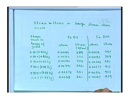
Let us take Fe 415 strain and stress, we shall get at this stress level 0.8 into 0.87 fy 0.00144 the strain, corresponding stress 288 let us give the unit 0.00163 306 at 0.9
