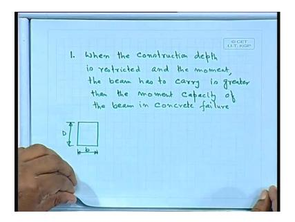
Now, let use comeback in few cases. When we have to provide the reinforcement, let use write down. When the construction depth is restricted and the moment, the beam has to carry is greater than the moment capacity of the beam in concrete failure. When construction depth is restricted and the moment, the beam has to carry is greater than the moment capacity of the beam in concrete failure.
