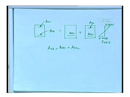
So, what is the design philosophy for doubly reinforced section? The design philosophy of doubly reinforced section; we shall provide the reinforcement in both sides. Let us say this 1 Asc: area of steel in the compression side and Ast: area of steel in the tension side. We can make in 2 parts; we can say that we are having a portion. This beam can take it a singly reinforced 1; that means, moment of resistance if we consider it as a singly reinforced section, only in the tension side.
