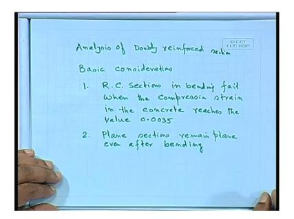
Now, let us come that your analysis of doubly reinforced section. We shall comeback for different other cases also, but before that let us take basic considerations. Number 1: RC sections in bending; RC sections in bending fail, when the compression strain in the concrete reaches the value 0.0035. We shall assume few cases 0.0035, that is, strain in concrete and here also it is valid in doubly reinforced section also.
