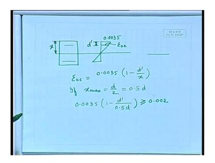
We have to find out the strain. The section we are providing here 0.0035, we have to find out epsilon sc in the strain in the compression side at the steel level, where we are providing the steel, that is, at a distance d dash from the top fiber, d dash from the top and we have x. What about epsilon sc epsilon sc? Will be equal to 0.0035 1 minus d dash by x; epsilon sc 0.0035 1 minus d dash by x. If, we assume if x maximum could we say d by 2, so we can write down d dash by 0.5 d.
