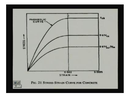
What we can do now, we are using this curve; it is dependent on the strain, upto 0.002 we shall come back upto 0.002 strain, beyond that we get constant stress in concrete, which comes as 0.45 fck. This portion less than 0.002 strains, we shall get that in a parabolic 1 we get the corresponding stress because, we have to find out the stress.
