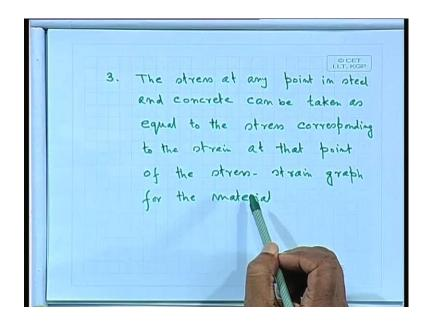
Number 3: the stress at any point in steel and concrete can be taken as equal to the stress corresponding to the strain, at that point of the stress-strain curve for the material. I repeat; the stress at any point in steel and concrete can be taken as equal to the stress corresponding to the strain, at that point of the stress-strain curve for the material. So, we shall get stress and strain, at a particular section that level we shall get the strain.
