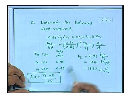
Step 2: determine the balanced steel required. We shall use the formula that 0.87 fy Ast, the steel has also reached the maximum stress equal 0.36 fck b times xu. We can write down it as Ast by bd equals 0.36 by 0.87 just rearranging times fck by fy times xu by d. Let use repeat Fe 250 Fe 415 Fe 500 xu by d 0.53 0.48 0.46 pt, what is pt? In other way, Ast? Ast equal pt times bd by 100.
