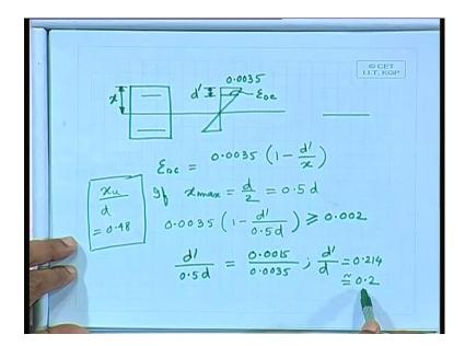
We are assuming if x max equal to d by 2 0.48 d xu by d for Fe 415, that we get 0.48. We can get it in is 456, we can also derive it also. xu by d equal to 0.48. That means, it is coming say reasonable assumption that 0.5 xu equal 0.5 d maximum. So, we can write down this expression, where it comes as d dash by 0.5 d equal to say 0.0015 by 0.0035. Therefore, I can write down d dash by d equal 0.214 approximately say 0.2. We can say
