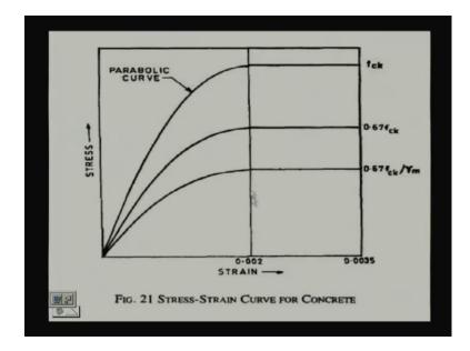
Our objective here; the strain where we are providing the steel reinforcement that d dash, if it is more than 0.002 the strain greater than 0.002 what we can get, we can always get 0.45 fck, we can get 0.45 fck.
