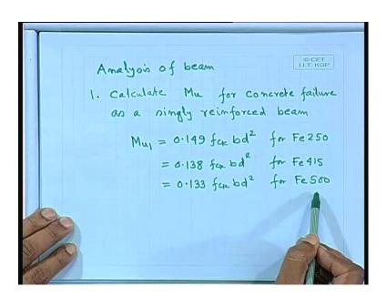
1: Let us elaborate the whole procedure. Calculate Mu for concrete failure as a singly reinforced beam. We can write down this part as Mu 1 equal to 0.149 fck bd square for Fe 250, equal to 0.138 fck bd square for Fe 415, equal to 0.133 fck bd square for Fe 500. We shall use the appropriate formula to get the moment of resistance for singly reinforced section, when the section is assumed to be failed due to concrete; concrete failure. Mu 1 for Fe 250 for Fe 415 for Fe 500.
