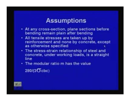
Let me just briefly tell that assumptions; yesterday I told the assumptions. So, let me just enlist it, related to that Working Stress Method. At any cross section, plane sections, before bending remain plane after bending. So, that means, actually your strain, the strain will be linear, that assumption, this assumption will be valid only when the strain is linear.
