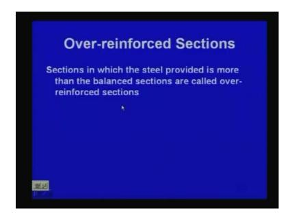
So, the other one is called over-reinforced sections. Sections in which the steel provided is more than the balanced sections, they are called over-reinforced sections. So, we shall consider this one as a over-reinforced section and under reinforced section. (Refer Slide Time: 13:41)
