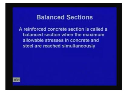
Before going to the calculations, let me tell you that what is a balanced section. Balanced sections, it means, a reinforced concrete section is called a balanced section, when the maximum allowable stresses, that means, sigma cbc in concrete, and sigma st in steel, so when the maximum allowable stresses in concrete and steel are reached simultaneously.
