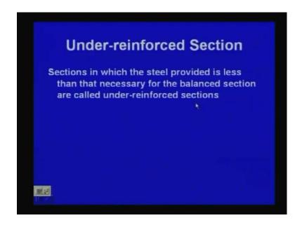
Next one we call it that under-reinforced section. So, that means, when the section is not balanced, so when the section is not balanced, we mean to say that it is also possible that related to steel I can say that, reinforcement steel, either that could be less or that could be more, because balanced is something that which is equal to the concrete strength.
