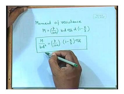
So, we can just repeat, moment of resistance; let me write down, moment of resistance, M equal to p by 100 bd sigma st d 1 minus k by 3. Also, you can write down in this way, m by bd square equal to p by 100 multiplied by 1 minus k by 3 sigma st.
