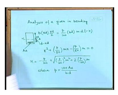
I shall come to the next point. We can find out, that analysis - one we call it design; another one we call it analysis. Analysis means that when the section is given, reinforcement, and the depth, width, everything given, then we call it analysis. Then we are analyzing that how much load it can take; what is moment of resistance.
