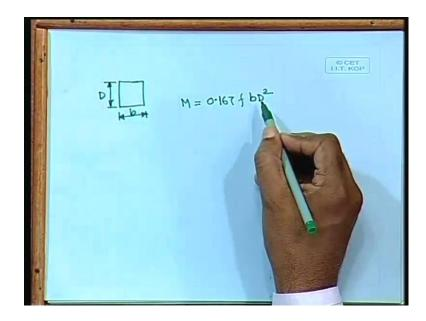
Just to recapitulate once more in this particular diagram. I repeat once more, D and b, and we have found M; M equal to moment of resistance we can consider 0.167 f b D squared. So, we can find out, say, the equation becomes very simple, handy, and we can find out the moment of resistance of that particular section. The section you are going to provide, if you know the moment, so you have to provide the moment of resistance.
