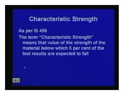
Now, let me find out in our IS 456, that our design code, what, how it is defined. The term characteristic strength means that value of the strength of the material below which 5 percent of the test results are expected to fail. That means, even if you consider a lot of say safety measurement all these things, even then also, that means, about 95 percent on the good faith, that way you can consider, and that is the value we shall consider our characteristic strength; that we shall consider.
