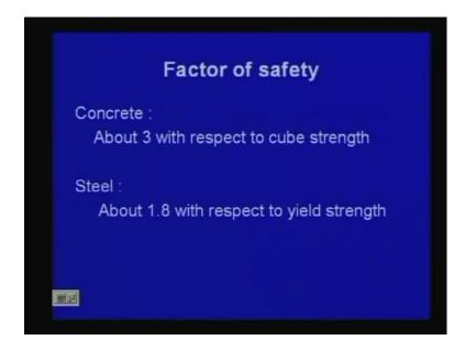
And we have to consider factor of safety. Factor of safety, we consider for concrete, about 3, with respect to cube strength. The cube strength that we have told, that cube strength, that cubes 150 by 150 by 150 - those cubes. So, from the cube strength, you will get it, that we shall find out, and we shall take factors up to 3.
