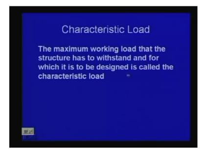
Similarly, we have the characteristic load also. The maximum working load that the structure has to withstand and for which it is to be designed is called the characteristic
