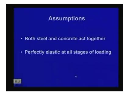
So, what are the assumptions? That both concrete and steel act together; it will work simultaneously; there is no slip; there is no slipping, that means, whatever you are considering that concrete and steel, the steel is embedded on concrete, and there is no slipping. Perfectly elastic at all stages of loading; it is perfectly elastic at all stages of loading - this one we are assuming.
