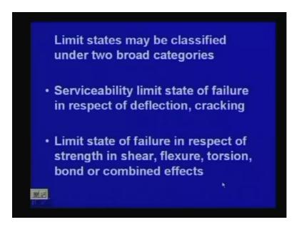
So, limit state may be classified under two broad categories. I have already pointed out. So, serviceability limit state of failure in respect of deflection, cracking. So, this is the one we consider is a serviceability limit state. The other one we consider limit state of failure in respect of strength, in shear, flexure, torsion, bond or combined effects that axial also will come, when we were talking, say your columns.
