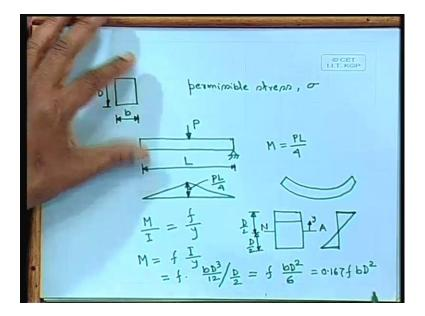
This is one, I can explain, this particular one, that we are considering, say, particularly, we are starting with the beam. We have to find out the dimension of say beam. If we have to find out the dimension of the beam, what we can do, let us forget the reinforced concrete for the time being; let us consider that we would like to provide a section, may
