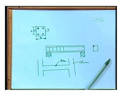
Only thing I would like to tell for this particular section here, we provide reinforcement, say if we reinforcement top also, that is you would get compression one; that means, in the compression side also you are providing reinforcement; in the compression side also you will provide the reinforcement.
