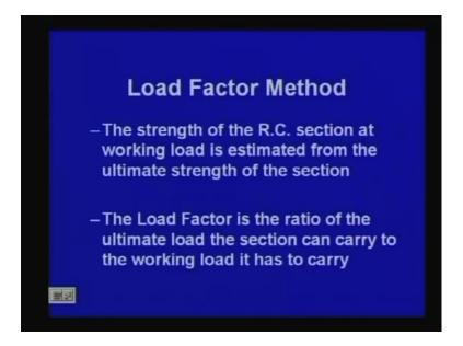
The strength of the RC section at working load is estimated from the ultimate strength of the section. So, we can find out the strength of the RC section, that one due to your working load, whatever load actually given, we can calculate from the ultimate strength of the section; we can find out from the ultimate strength of the section; that means, we
