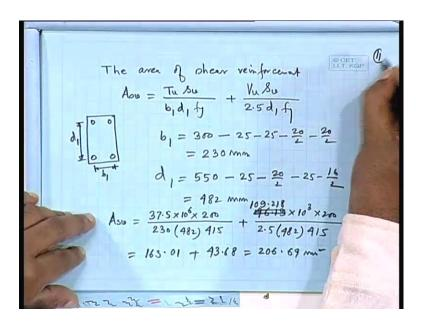
So, let us do 1 by 1 then so 37 5 10 to the power 6 into 200 divided by 230 divided by 482 divided by 415, which comes as 163 01 say plus 109 218 10 to the power 3 into 200 divided by 2 5 divided by 482 divided by 415 which comes as 43 68. So, this 1 equals 163 01 plus 43 68 206 69 square millimeter.
