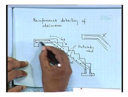
So, distribution steel will be according to that 0 12 percentage of that for the slab, for slab that is 0 12 percent. Here I would like to say, that for slab that is 0 12 percentage for the tor steel, for beam it is 0 85 by fy. Now, where you are providing any stirrups or shear reinforcementwe can treat it as a slab. So, that means there we shall provide say 0 12 percentage, but where we are providing that your say stirrups.
