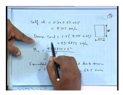
So, after few iteration few trials we have come to the section that is having that width of the beam that is 300 millimeter and overall depth that is 500 millimeter. So, I think not 550 so 300 by 550 that is the over all depth. So, the self rate that we have got it as 4 125 kilo newton per meter design load with that factor 1 5 4 125 plus 25 which comes to 43 6875 kilo newton per meter. That ultimate moment parallel due to the simply supported beam we are getting 136 52 kilo newton meter.
