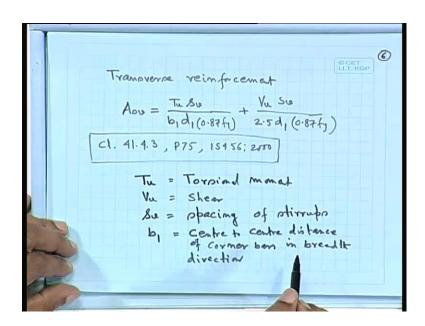
There is one more thing that is your say for transverse reinforcement, that is your say shear reinforcement. We find out here say Asv that your say stirrup that area of stirrup or reinforcement it says Tu by Asv; Asv the spacing of stirrups or web reinforcement b1 d1 times 0 87 fy plus Vu Sv divided by 2 5 d1 times 0 87 fy. We can find out the area of steel using this formula in clause 41 4.3, page 75, IS 456: 2000.
