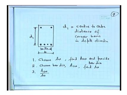
If this is your beam so, we are having reinforcement so b1 means there are many so many bars b1 means this is your b1, along breadth direction b1. So, what about d1? Along the depth direction. So, b1 will be equal to b if this is your b so b minus that clear cover this side 25 millimeter, clear cover this side 25 millimeter minus that half of the diameter here; half of the diameter so that means, 1 diameter.
