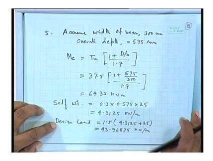
So, assume width of beam say 300 millimeter, overall depth 575 millimeter here since I have changed the 300 I could reduce it or anyway let us, do not change this. Because, it
