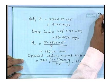
So, 0 3 times 0 55 times 550 times 25 comes as 4 125 kilonewton per meter design load equal to 1 5 times 4 125 plus 25 equals 43 6875 kilonewton per meter Mu equal to 43 6875 times 5 square divided by 8 equals 136 52 kilonewton meter equivalent moment so, 37 5 1 plus 550 by 300 by 1 7 equals 62 5 kilonewton meter. So, this is due to torsion only this is due to torsion only.
