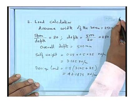
So, step 2 say load calculation we shall try say few trials. Because, instead of directly going to the value it is worth that going say all the calculation because; what are the process, how we repeat the whole calculation. let us start like that. Because, I do not want to make the final value and see that as if it is a magic way we have got it but, it is not like that when we are designing then we do lot of say you are repeating steps.
