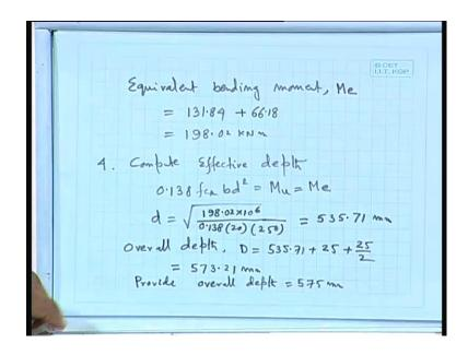
So, what about the equivalent bending moment? equal to 1 31 84 that is the Mu we have got it due to the applied load plus equivalent moment, which is coming as 66 18 and which is coming as 198 02 kilonewton meter. So, what about the effective depth we can compute we can check effective depth let us compute effective depth. So, we have the same formula so 0 138 fck bd square equal to Mu.
