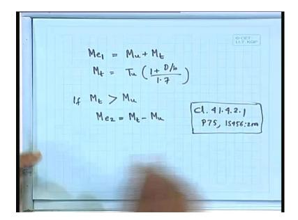
So Mt minus Mu that means, say let us say I have told Me1 equal to Mu plus Mt, where Mt equal to Tu 1 plus d by b divided by 1 7 and this is one case. The other case is that, if Mt is greater than Mu then I shall take Me2 will be equal to Mt minus Mu. So, this is other case and for that we have to provide the reinforcement at the top, we shall provide the reinforcement taking Me2 equal to Mt minus Mu.
