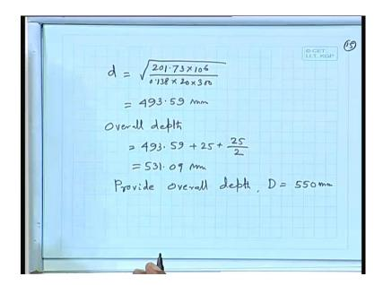
D equal to let us calculate d. So let us you see that 493 millimeter only, overall depth 4930 59 plus 25 let us still take 25 millimeter dia bar we shall provide. So, 531 09 millimeter provide overall depth D equal to say 550 millimeter 540 also we can provide but, anyway let us say 550 millimeter.
