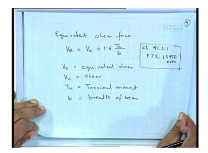
So, what is the that what our code says this is very simple one we can say for equivalent shear force. So, we can say in a particular section we can say Ve, where that torsion is acting. So, Vu the shear force from the usual whatever way you have got it plus 1 6 Tu by b. This one available, in clause just for your reference clause 41 3 1, page 75, IS 456: 2000.
