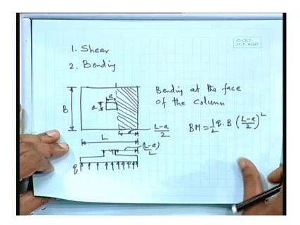
That we can do it, but before that let us take that we have shear and bending we take it say if this is the plan of the footing. The bending we consider at the face of the column. So, bending we shall consider at the face of the column. That means, if this your length L, this is your say B, a is the say column and let us take this is square. So, this length is equal to L minus a by 2 so that means, we shall take this portion L minus a by 2.
