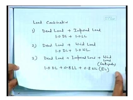
Then, what should be your loads it should have load combination: number 1 dead load plus imposed load. So, it comes please note for calculating size of the footing for size of the footing we do not take that 1.5. Because, we are noting the limit state rather, we are taking that 1 say working stress. Because, the bearing capacity of the soil is given as say you are working stress that 1 that serviceable 1, not the 1 limit state or ultimate bearing capacity.
