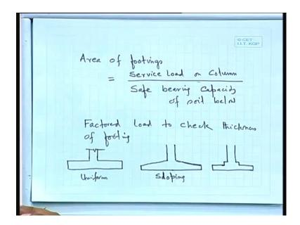
So, what should be the now come back to the area of footings we have to calculate. So, service load on column divided by safe bearing capacity of soil below. So, if we know the service load that means, giving the proper multiplication factor 1.0 this case or 0.8 with the live load and the wind when you are talking. So, service load on column divided by say bearing capacity of soil whatever there on the basis of that, you can get the area of footings.
