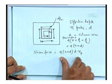
It means, if this is a column position. So, we shall go all along in all side and this 1 will give you at a distance d by 2; d is the effective depth of footing. What does it mean? What we are doing basically? We are doing here because, punching means simply it will piers that means, as if this portion we are applying load like this. That means, as if this portion simply break and it will just simply insert that 1.
