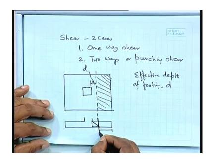
Next 1 we shall get it so that shear, we have 2 cases: 1 we call it 1 way shear, the other 1 is called 2 ways or punching shear. What about this 1 way shear? 1 way shear means, if this is the column position if effective depth of footing d. Then, we have to take a section at a distance d. So this your d that means, shear force we have to compute where this section compared to the bending moment.
