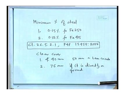
So, what about the minimum percentage of steel? In this case, we shall use that slab that whatever we provide the minimum reinforcement for slab that is 0.15 percent for Fe 250 and 0.12 percent for Fe 415 and these we will get in just for your reference clause 26.5.2.1 of page 48 IS 456: 2000 the same clause for slabs. What about your cover? Generally, we provide say 40 millimeter not less than 40 millimeter.
