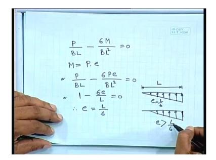
So, if we write down here P by BL minus 6M by BL square equal to 0. So, what shall we get here M equal to P times e the other way I can write down M equal to P times e. So, I can write down or. So, equal to e equal L by 6 that means, if we get e equal to L by 6 in that case what will happen, it will happen that you will get only on 1 side. That means, if this is the length L of the footing so, in 1 end we shall get 0.
