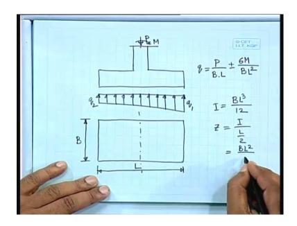
Let us, say the load applied P and moment say M and the plan of the footing let us, say this B that width and this is length L. Since, we are having moment here so, we shall get it will not be uniformly stressed since, we are having moment. So, because of that we shall if we have axially loaded 1 then, we shall get uniform all along. But here since, we are having moment what we shall get we may get something like this.
