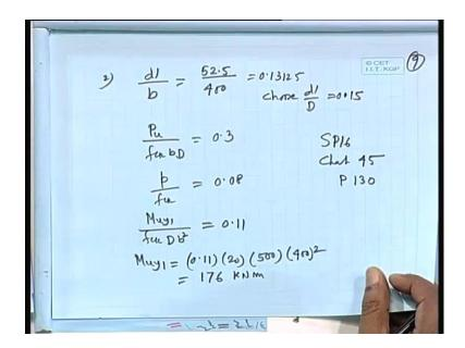
So, SP16 chart 45 page 130 and this is 0 11. So, Mu y1 equal to 0.1 times 30 times 500 times 400 whole square. So, let us check 176 shall I accept it 176 kilo newton meter right. So, Mu y1 that is say 100 and 176 kilo newton meter. So, we know Mu x1, we know Mu y1 what about Pu z?
