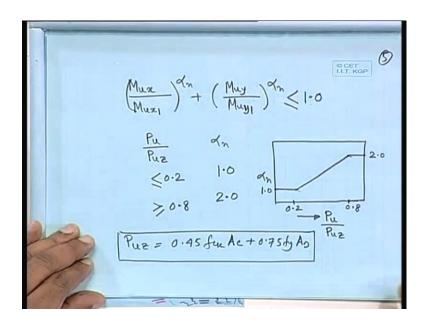
The check is Mu x by Mu x1 to the power alpha n Mu y by Mu y1 y1 times alpha n should be less than equal to 1.0 what about this I know Mu x that is given for that I have to design, I know Mu y for that I have to design. And Mu x1 I have got it from the proper chart with d dash by d fy all of them I have got Mu x1, I have got Mu y1, but I do not know alpha n, what is that alpha n? Alpha n is dependent on Pu by Pu z I have already computed Pu z.
