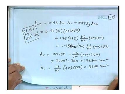
So, Pu z equal to 45 fck Ac plus 0 75 fy Ac equals this 1 you will get it again clause 36 9 page 71, IS456: 2000. So, 0 45 times 20 times 400 times 500 plus 0.75 times 415 times p how much you have chosen p equal to 1.6. So, 1 6 by 100 times 400 times 500 so, this much is your area of steel we are getting it here and we should not stop it here.
