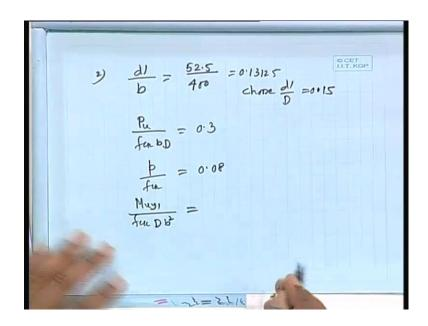
So, number 2 d dash by b will be equal to 52 5 divided by 400 because, so, I am taking about the other axis. Let us, say that is the minor axis so 52 5 divided by 400 0 13125. So, choose d dash by d equal to 0 15 I shall take that chart, where d dash by d equal to 0.15 Pu by fck bD there you no problem, it will be same 0 3 only there no change p by fck also there is no change 0 8 Mu y1 by fck bD squared that 1 we shall get it. And where from we shall get it, we can get it from the chart 45.
