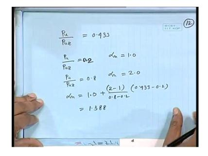
So, Pu by P uz we have computed 0.433 for Pu by P uz equal to 1.0 alpha n 0.2 this is 0.2 alpha n equal to 1.0 Pu by P uz equal to 0.8 alpha n equal to 2.0. So, alpha n equal to 1.0 plus minus 1 times 0.433 minus 0.2. So, how much is coming so, 0.233 divided by 0.6 plus 1 so 1.388 .So, we have got that alpha n equal to 1.388. So, let us now summarize the thing.
