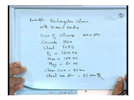
So, let us take the column section size of column 400 by 500 concrete M20 steel fe 415 Pu let us, take n 1200 Mu x let us take 100 kilo newton Mu y let us, take 8 kilo newton clear cover 40 millimeter. So, and we shall let us try 20 millimeter bar steel bar dia so, what we can do it here d dash by d let us compute.
