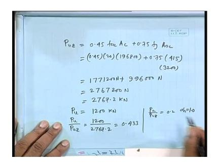
Pu z I have calculate so, 0.4 fck times Ac plus 0.75 fy Ac equal to 0.45 times 20 times 196800 plus 0.75 times 415 times 3200. So, 0 5 times 20 times 196800 175 times. So, 1771200 plus 175 times 415 times 3200 9960 these are all in newton. So, last 1771200 2767200 newton which comes as 2767 2 kilo newton. So, P uz equal to 2767.2 kilo newton what about your Pu equal to 1200 Pu by P uz equal to 1200 divided by 2767.2 equals 0.433 alpha n alpha n equal to 1. Let me, do it in the next page.
