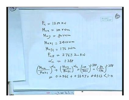
So, what we shall do it here Pu 1200 let me come to that portion, where I have missed those values yes. Pu equal to 1200 Kilonewton Mu x equal to 100 Kilonewton Mu y equal to 80 Kilonewton Mu x1 how much you have got Mu x1, 240 Kilonewton meter this 1 all meter Kilonewton meter and Mu y1 176 Kilonewton meter again I am out of paper Mu x1 Mu y1 and P uz 2767.2 kilo newton. So, we can add alpha n computed equal to 1.388.
