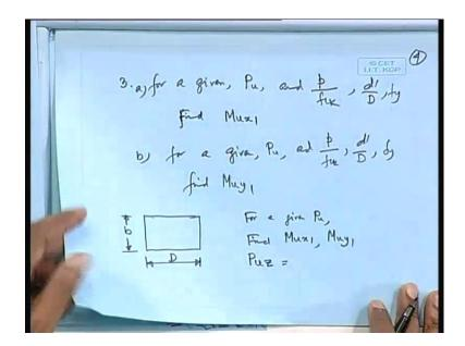
For a given Pu and p by fck, find and also d dash by d find Mu x1 what does it mean? It means, that Pu is given I have already chosen p by fck and also I know d dash by d that means, I can go to a since I know p by fck d dash by d also, I know fy; fy is the that steel grade. So, since I know Pu, p by fck, d dash by d fy. So, I can go to proper chart of sv 16 and then, what I can do since I know Pu.
