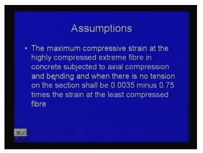
The maximum compressive strain at the highly compressed extreme fibre in concrete subjected to axial compression and bending that means, axially loaded. As well as bending also there and when there is no tension on the section shall be 0.0035 minus 0.75 times; the strain at the least compressed fibre.
