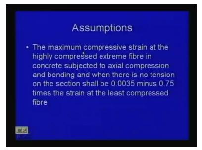
It says the maximum compressive strain at the highly compressed extreme fibre, in concrete subjected to axial compression and bending and when, there is no tension on the section shall be 0.0035 minus 0.75 times the strain at the least compressed fibre. So, let us draw the cross section, I think let us make it; so, we can have this is the cross section of a column.
