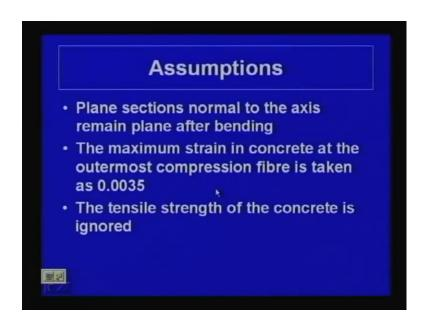
What are those? That plane sections normal to the axis remain plane after bending. The maximum strain in concrete at the outermost compression fibre is taken as 0.0035 so, that is the limiting strain for concrete. The tensile strength of the concrete is ignored just let us recapture it once more.
