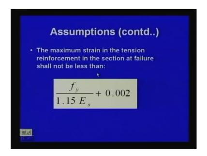
The maximum strain is dependent on the steel used. So, from there we can find out the maximum strength that for say Fe 415 or Fe 250 or Fe 500 we shall get different limiting strength for steel.
