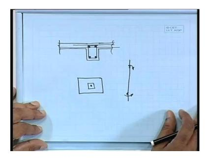
So, if it what I mean to say this is your beam say slab, this is your beam let us say. So, your reinforcement is going up to this for beams and here whatever, your reinforcement for the slab that is also there, if not that we are not concreting here. Because, it will be cost materially with the slab also so, and you can see few places there is a lapping big 1, small 1 all those things.
