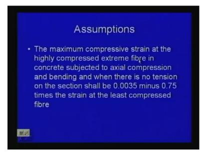
Now, the maximum compressive strain at the highly compressed extreme fibre if it let us, read it. Because, this is very important the maximum compressive strain at the highly compressed extreme fibre in concrete subjected to axial compression and bending subjected to place, not axial compression and bending. The past 1 I have told that is direct compression only fcl load while you are limiting strength 0.002 and the stress will be 0.45 fck.
