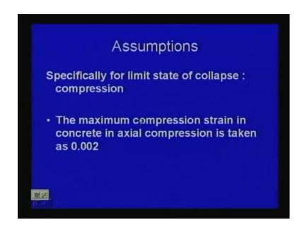
Now, specifically for limit state of collapse: compression in addition to those the maximum compression strain in concrete in axial compression is taken as 0.002. That means, we are talking that 0.0035 8 that 1 that limiting strength that is for from the
