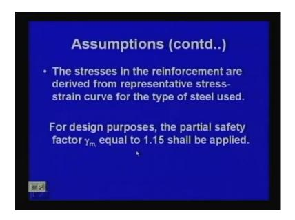
The stresses in the reinforcement are derived from representative stress-strain curve for the type of steel used. For different steel we have to use different your stress-strain curve.
