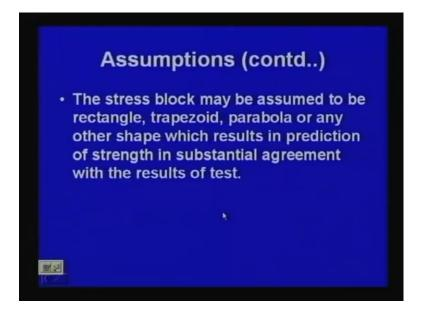
The stress block may be assumed to be rectangle, trapezoid, parabola or any other shape which results in prediction of strength in substantial agreement with the results of test. This is the 1 that already, we have taken care of that which type of say your stress block we have to use.
