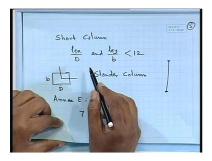
So, it means here if I go back to the previous 1 it means, the effective length should be if it is fixed then we have to find out suitably that lex and ley from the length whatever given. We can find out lex and ley then, we can divide by the D; that means, in the other way it will govern us to find out the D also. Because, if I know the le effective length then, we can find out what should be the dimension?
