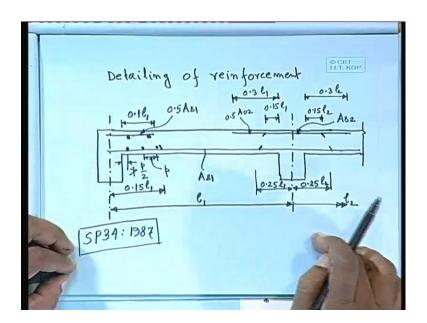
Let us start with the detailing, because last class I have not finished that part. So, detailing of reinforcement that is very important. So, I shall just tell you very few things that which we should know. Let us say this is beam cross sorry slab cross section and let us give a centre line and we have the length 11 and other part we can specify like this that
