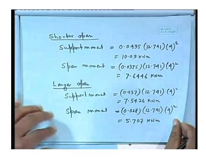
So, shorter span support moments 0.0495 times 12.741 times lx 4 square which comes as 10.09 kilo Newton meter span moment, in the shorter span we can get it 0.0375 times
