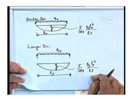
So, we can write down. So, if this is your lx. So, as if we are having 1 beam or whatever we consider a plate qx and this is the span that 1 we are getting say your lx. So, you can write down the displacement 5 by 384 q lx to the power 4 by ei this is your that vertical displacement. Similarly, this is shorter deduction. The other 1 longer deduction in the similar fashion you can write down. So, this side you have the UDL qy and we have the vertical deflection and this is your ly.
