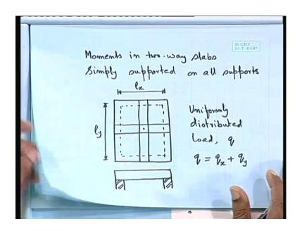
Now, let us come to the 1 case that moments in 2 way slabs special case say simply supported on all supports please note the supports are on yielding that supports, will not be deflected this is a 1 case I can say as if we are having the slab which is supported over brick wall in all 4 sides. So, brick wall in all 4 sides and we have to design that we have to find out that moment distribution; that means, whatever the load we are getting here may we can say uniformally distributed load.
