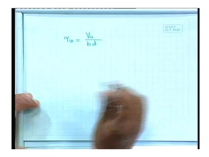
So, vu is the design force. So, tow v equal to vu by bd that is the nominal shear stress. So, vu we are getting from our calculation after giving the proper factor all those things. Vu we know that width d all ready we have given that d because depth of the section all ready we have done it for the flexure point of view. So, i can get tow v.
