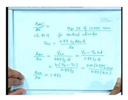
So, we can write down asv, asv by sv equals we can write down asv by sv equals we have already noted down we can go to that. So, for vertical stirrups as per our code says we can write down here. Let us write down first clause forty point four for vertical stirrups. So, which comes as it says. Vus equal to 0.87 fy asv times d divided by sv. So, you can write down this 1 and this is given in page seventy three of is four five six.
