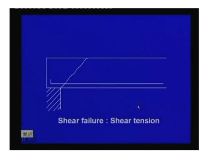
The shear failure we can have different types shear failure this is due to say shear tension this is 1 case this could be due to shear tension.
