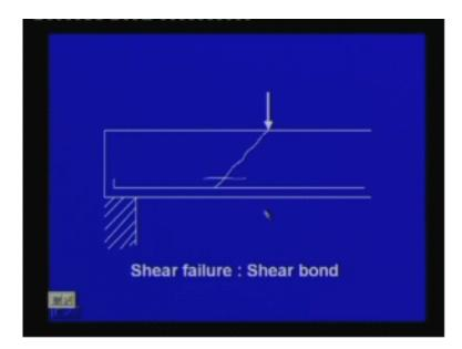
We can have that is 1 the shear bond apply load here and that is a shear bond that also you can resist.
