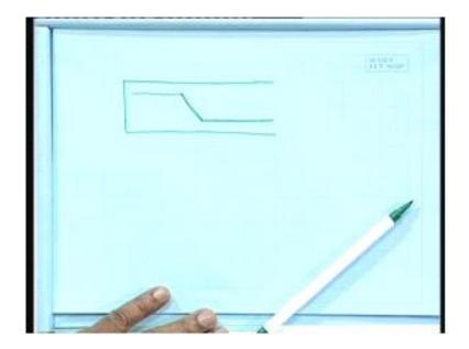
This is your say beam what we can do if we take say simply supported beam generally say simply supported beam that when you are in 0 that in the support. So that means, we do not need that much of tension your say tensile reinforcement. What we can do the bar which is coming from this side the bar which is coming from this side. Because, that we are assuming the tensile force that tensile is in the bottom in the most of the cases.
