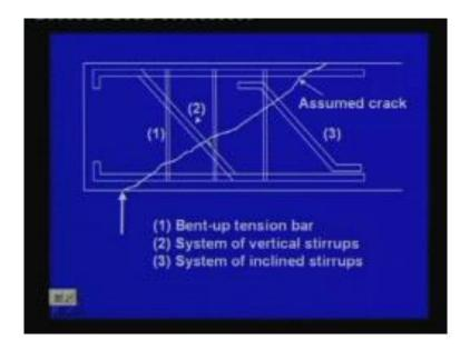
This is 1 bar this is 1 bar. So, then this bar is coming from this side then it is bent going upward and then this way. So; that means, it will also resist certain portion or part of the shear. The second 1 system of vertical stirrups the system of vertical stirrups means these bars which we have to provide. And the third 1 system of inclined stirrups the stirrups also we can provide in the inclined manner in this fashion.
