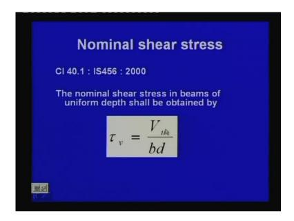
So, here that vu the force, so vu the shear force that is the design shear force divided by b that width of the beam and d that is the effective depth. So, we shall get the shear stress tow v we shall get the shear stress tow v that our code says that do not go for that parabolic distribution all those things. So, we can take the nominal shear stress and we shall we can do our calculation.
