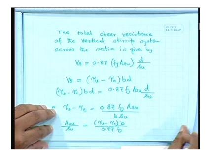
So, we can find out here the total shear resistance of the vertical stirrup system across the section is given by vs equal to 0.87 times fy asv times number of stirrups d by sv. This we have all ready have done. So, 0.87 fy asv is the for the 1 say stirrup which is say it may be 2 legged 4 legged that which taken care of any asv times. That number of stirrups that spacing on the basis of that we have already done say n, so, d by sv.
