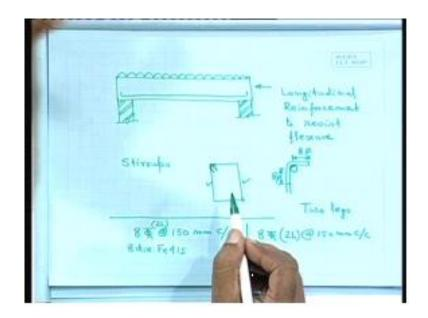
We use tie or we use stirrup. How it looks likes? The stirrup is made this way; that means, you take a bar and you start bend. So that you can make this type of thing and generally it comes generally it comes. If we take the bar which can come and this 1 the longitudinal 1 we are looking from this side we are looking from this side. So, this is your longitudinal bar and from the central line of longitudinal bar which will come in the range of say 8 phi 8 times the diameter of this stirrup.
