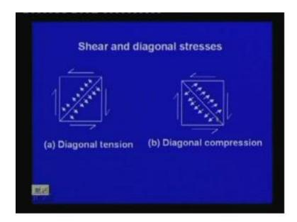
So, you can have the diagonal tension if we take 1 element and you can have diagonal tension. So that, the crack it will just split and other thing also possible it should be the other way the diagonal compression. So, I think it should be the other way in this particular one. So, we can have the diagonal compression and similarly we can have tension in beams.
