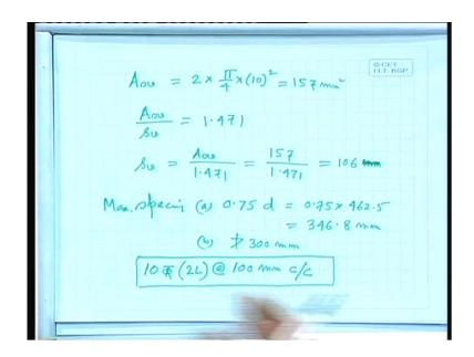
So, asv equal to 2 legged 2 into pie by 4 let us take 10 millimeter because we can do trial and error let us take i am taking say ten millimeter. So, which comes as 157 square millimeter asv by sv. We have already computed as 1.471 sv equals asv by 1.471 157 divided by 1 471 equals 106 square 106 millimeter. So, what about the spacing maximum? So, let us say maximum spacing point 0.75 d equals 0.75 times how much is your d.
