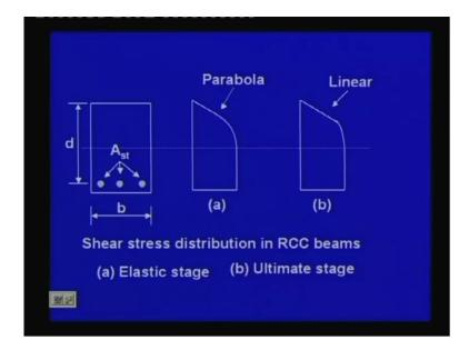
Now, what about the shear stress? The shear stress distribution for rectangular section it comes parabolic in the elastic stage say we are getting in this pattern, ultimate stage that these portion becomes linear. But in our calculation, but in our calculation we shall not use this formula what we shall not use this stress distribution. What our IS code says let us find out.
