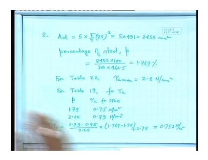
Number 2 ast the area of longitudinal steel ast 5 times whole square equals 5 into 491 which comes 2455 square millimeter. What about then percentage of steel p equals 2455 into hundred divided by 300 into 462.5 that effective depth equal to 1.769 percent. From table 20 tow c max maximum tow c max equal to 2.8 Newton per square millimeter. From table 19 for tow c. P 1.75 tow c for m 20 I am just giving the part from table 19. So,
