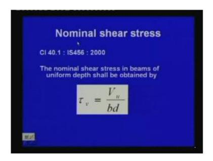
So, we shall take care that nominal shear stress according to is 456 that our code says that we are shall not go to that parabolic distribution. In a state we shall take this nominal shear stress and we will find out in this clause the clause 40.1 IS 456 2000. The nominal shear stress in beams of uniform depth shall be obtained by tow v, that is the shear stress developed equal to vu; vu is the design shear force vu is the design shear force.
