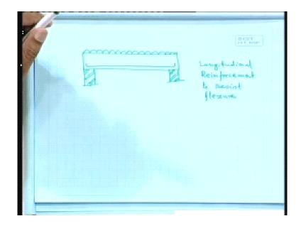
So, let us take a simply supported beam resting over a brick wall. If we have uniformly distributed load let us apply the uniformly distributed load. We have the bending moment to resist bending moment. What we have to provide? We have to provide longitudinal reinforcement. This is for longitudinal reinforcement to resist flexure or bending. In addition to that you can have that shear and diagonal stresses you can have shear and diagonal stresses.
