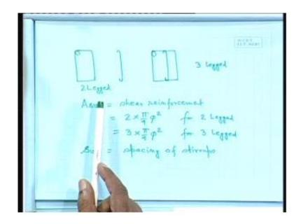
And the different types of bars that stirrups could be 1 simple 1 that what we generally provide this 1. If we need more then we can have single link like this also; that means, we are providing the reinforcement say and this bar will come like this. Then we shall consider this 1 as 3 legged whereas, this 1 2 legged. So, asv the area of steel if we designate. So, far we have done ast the tensile reinforcement longitudinal 1 and here we specify as say asv this is your shear reinforcement.
