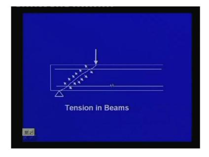
That if we take, these are the longitudinal reinforcement. So, it can have tension. So, this is and we have 2 that we have to resist these cracks and how shall I how shall we make it.
