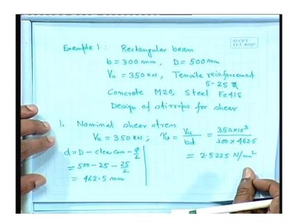
So, what we shall do let us take 1 example. Let us take the rectangular beam b equal to 300 millimeter D equal to 500 milli millimeters. Vu 350 kilo Newton tensile reinforcement please note tensile reinforcement. I am repeating every time tensile reinforcement not the compression because that table 19 of IS 456 it gives on the basis of
