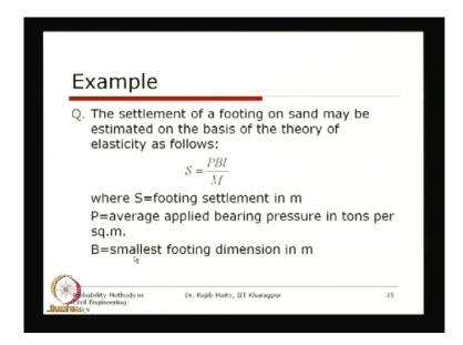
One small example we will take - the settlement of a footing on the sand may be estimated on the basis of the theory of elasticity as follows s equals to p b i by m - where s is the footing settlement in meter. P is the average applied bearing pressure in tons per square meter and b is the smallest footing dimension in meter.
