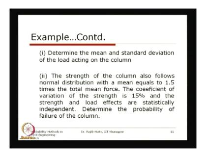
Now, the, and the second question is that the strength of the column also follow a normal distribution with the mean equals to the 1.5 times ofthe total mean force and the coefficient of variation on the strength is 15 percent, and the strength and the load effects are statistically independent determine the probability of the failure of the column.
