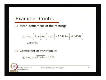
Andthe mu of this means settlement of the fore footing as you know from this log normal distribution is from this expression, we just refresh this lambda and sigma s this. So, this will the mean settle will be the 0.0, 0.092 meter, and the coefficient of the variation which is approximately equal to the sigma s and which is 0.2131.
