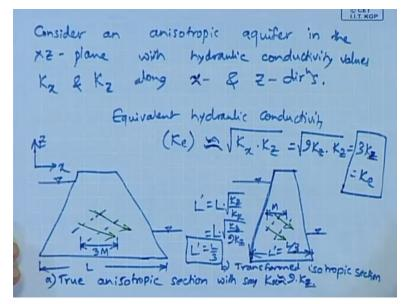
Now let us consider and isotropic case where in say consider in an isotropic aquifer so here which as a in the XZ plane with hydraulic conductivity KX and KZ along X and Z directions and typically in case of the alluvium or aquifers so this KX will be greater than the KZ.
