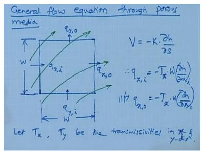
And so this regarding the now let us consider let us go to the general flow equation through porous media so here let us consider through two dimensional flow initially and again later on let us extend it into a three dimensional level flow domain. So in this case this is the flow domain two dimensional flow domain and then say these are the stream lines shown by this green color and let considering the unit width let the flow across the this boundary of this square flow domain the QXI.
