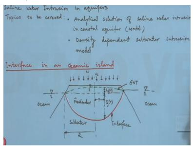
So this is pure lecture number 33 and in this one we will talk about Saline water intrusion in aquifers and topics to be covered are first one as analytical solution of Saline water intrusion in coastal aquifer we will continue from previous lecture class next one is density dependent salt water intrusion model we have already talked about salt water intrusion in confined and unconfined aquifers.
