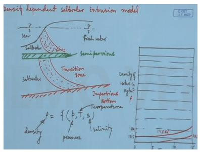
So next thing we will discuss is this density dependent flow models what is this density dependent density dependent salt water intrusion model so in this model a transition zone is considered in state of a sharp interface that is used for our sharp interface modeling using Herzberg principle let us say we have some semi pervious semi pervious location and we have another.
