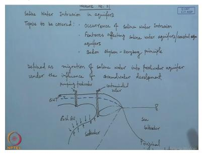
So this is lecture number 31 and our main topic is saline water intrusion in aquifer and topics to be covered under this particular lecture class are occurrence of saline water intrusion. Second are features affecting saline water aquifers or coastal aquifers and third one is BODON GHYBEN HERGEBRG principle.
