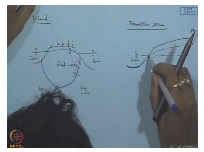
Another situation we can have that is island situation that is for island aquifers fresh water interesting for island aquifer. We have different settings which on the top we have fresh water and from the bottom we have this saline water and this is our normal ground water table and in islands only source of water are fresh water is natural recharge natural recharge is the only source of water.
