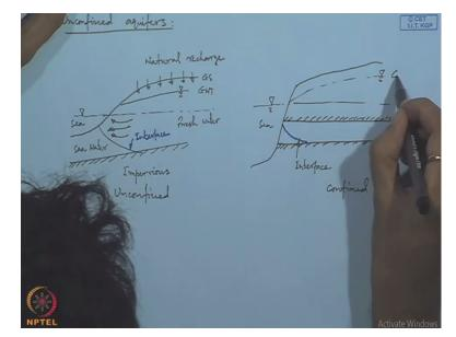
So if we distinctly see different things so for unconfined and confined aquifers for unconfined aquifers we can have different situations first one is your bate condition which is impervious in nature. Then this is sea level and natural recharge or natural recharge is offering from the top this is our ground water table GWT this is our GS our ground surface.
