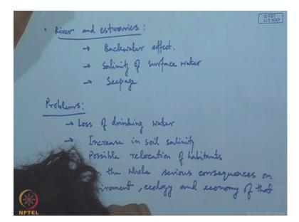
And last point under this particular thing is effect of river and Estuaries River and estuaries one point we can say that is backwater effect salinity of surface water and final thing is seepage. So what is this backwater effect due to these rivers which are connected to the sea there may be backwater effect and due to tidal variation it can affect significant portion of the river.
