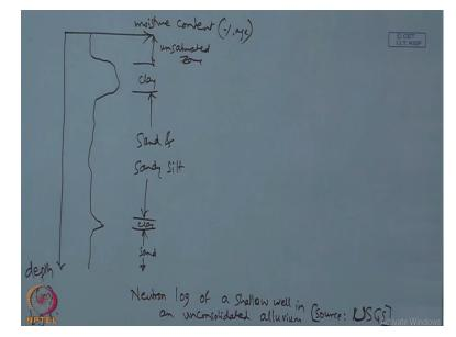
And here there is one a typical neutron log so here this is the depth in meters below the below ground level. And this is the moisture content in percentage so this is neutron log of a shallow well in an unconsolidated alluvium. So this is taken from the US geological survey and here so the so based on this we can say if the moisture is more so then we can say it indicates a clay.
