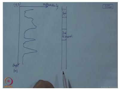
So these are the application and in this a typical natural gamma ray log will has a depth along the vertical axis. And then the radioactivity along the horizontal axis an here so in this case so this will constitute something like this. And here so this is 0, 0 and this corresponds to so in the geological log so may be this corresponds to sand.
