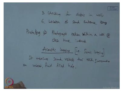
Then the third one is checking for debris in wells and location of sand entrance zones. So there is also what called photo log is so this photo log so it is basically photographs taken in a well that is within a well at close time intervals. So this is regarding the TV logging next we will go to what is called the acoustic logging.
