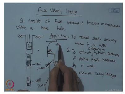
So next we will go to the fluid velocity logging so in this fluid velocity logging so it consists of fluid movement tracking or measurement within a bore hole. So its applications to reveal strata contributing water to a well to estimate the hydraulic differences. So estimate differences in hydraulic parameters of various aquifers intersected by a well and thirdly to estimate casing leakages the leakages in the casing in pipes.
