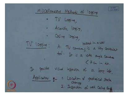
So in this there are this TV or say television logging there is acoustic logging and the third one is the casing logging. So these are the three important techniques which are grouped under the miscellaneous logging. And here so this is now let us come to this TV logging so this is in this a TV camera television camera is a very convenient tool.
