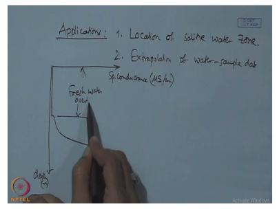
And the applications so the applications are one is the location of saline water zone two is extrapolation this fluid electrical the conductivity log can be used for extrapolation of water sample data and. In this case say for example a typical fluid conductivity log it will have so the depth in meters and then the specific conductance in micro siemen per centimeter.
