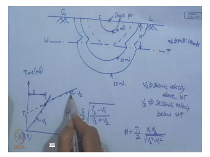
So in this case first let us draw the figure and so this is the ground surface. And here you have the shock point and the waves expand outward from the shock point. So this is the shock point and so here this is the water table so this is at distance of H below the ground. And here so this is the time is in 10 milli seconds.
