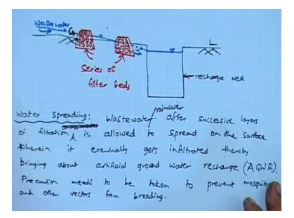
So here we can a typical diagram you can show say suppose this is a recharge well and of course here I am showing this as a an open well and so this is the waste water and so typically so different kinds of so this filter beds are employed and so here we can may be another and in this case so this is the recharge well so this is the this is the ground level so this is the waste water.
