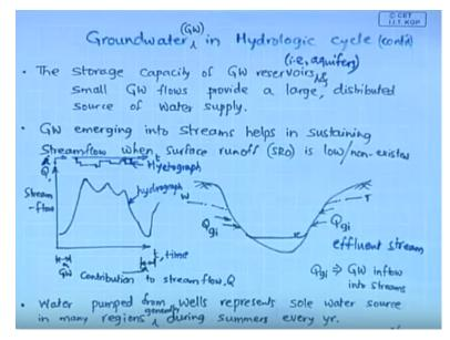
And here let us go to this one so the ground water is stored in the below the ground in water barring layers which are known as aquifers. So this storage capacity of these reservoirs so that is which are commonly referred to aquifers as well as the small ground water flow because when these aquifers gets saturated.
