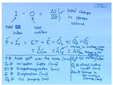
So can be written as I - O = Delta S / Delta T so this is the ground water inflow or let us say this is total inflow and this O represents the total outflow and this delta S / delta T represents this total change in storage volume. The same thing we can write it as this as P + IR = ET so here the P represents let me write all this P represents the precipitation.
