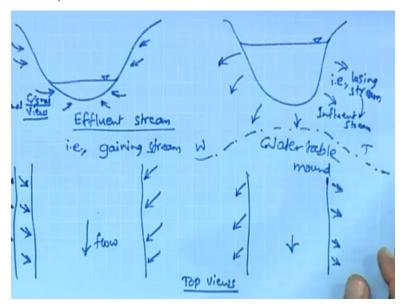
I mentioned type of stream which is known as the effluent stream so this is the effluent stream in this case there may be contribution from the bed as well as banks into the stream. And this is also referred to has a gaming stream similarly there are another type of stream which is known as a losing stream. Wherein this stream is having a high water level and then so because of this there is infiltration from the stream into the ground and this is they refer to as the water table mount.
