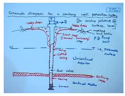
And here so this one so schematic diagram for a sanitary well protection system and here say the so in this case systems a safe or a existing pollutants at surface level of course this is reasonable simpler but if the pollutants are existing at the subsurface level then it makes it much more complicated. So in this case so here let us so this is the ground level of course here it is generally wells they may not have this kind of poor mount.
