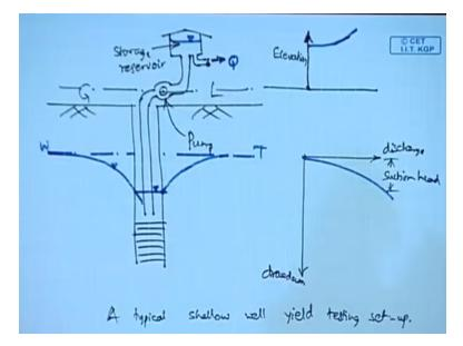
In this case it typical so this is the ground level and here we have the well and here we have the pipe so through which so this is a storage reservoir. So this is a here you can say this is the water supply this one so this is a storage reservoir and then this is the pump and then this is a ground surface and then the static water table. So here this is the water table and after this pumping so the so there will be a formation of cone of depression and this is this one.
