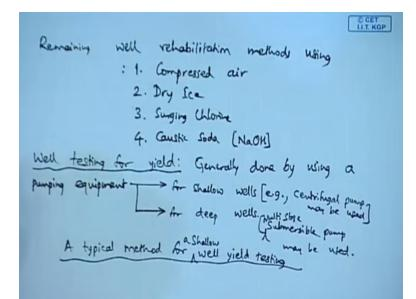
So the remaining well rehabilitation methods using it is one compressed air two that is dry ice that is obviously solidified carbon oxide and then third is a surging chlorine and followed by lastly caustic soda that is a NAOH. So these are also used this one so the so this will complete this rehabilitation and of course for want of time are not able to give much this one and next we will go to that is the well testing for yield.
