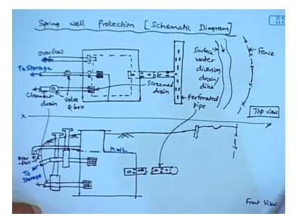
In this case it is let us say schematic diagram so in this case so let me so draw this is the top view and then so here let me draw from view. So in the top view so essentially we have so there is a and overflow pipe so this is overflow so you may want to denote this one. Next there is storage so there is also another pipe which takes to storage so this is to storage.
