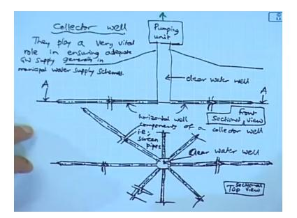
Now let us consider the collector well and this case suppose this is the suppose this is the top view and here this is the of course here if you want again there can be a break line. So this is the pumping unit so through which the water is pumped so this is the sectional view section front view. So these are so it is horizontal wells horizontal well component of a collector wells.
