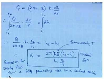
So in this we will get the expression for the steady rate of pumping so this Q is simply given by 2PieR into B so this is the area of flow for the radially inward flow into K into DH / DR. So this is the area multiplied by velocity that will give the expression for the steady flow rate into this well. So therefore let us rewrite this terms so this Q / 2 PIE KB into DR / R this = DH.
