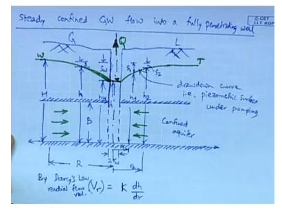
Let us consider steady confined ground water flow into a fully penetrating well in this case the well is penetrating for the entire depth of the confined aquifer. So let us draw the sketch here so this is the bottom impervious layer of the confined aquifer and here so this is the well. In this case let us say this is the top confining layer of this confined aquifer and obviously so here the strainers basically well casing with perforations and so this is the confined aquifer.
