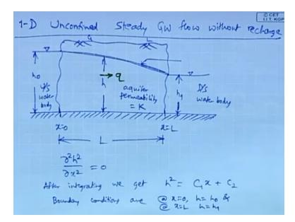
Now let us come to this another case that is the 1D unconfined steady ground water flow without recharge. So here we know that so in this case so let me draw the figure here in this case this is the bottom confining layer for the unconfined aquifer and then there is upstream water and then this is the general ground here and then there is a downstream water body.
