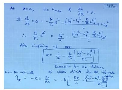
So we know that at  $X = A H = H \max DH / DX = 0$  so this is the condition for maximum. So therefore let us differentiate this expression so that is 2H into DH / DX this is equal to so this and let us substitute because this is DH / DX which is 0. So therefore we are equating it to 0 and then the right hand side and that in place of X we have to substitute the value of A.
