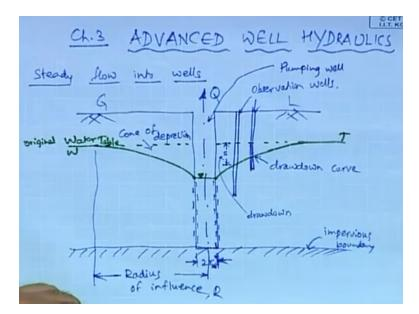
So the discharge per unit width so that is Q so this is = -KH DH / DX so this is = -K and X into DH / DX is simply given by it is H1 square – H0 square divided by 2L into so that is the H into DH / DX. So therefore the discharge per unit width so this is the expression for so this is the expression for the discharge per unit width. So for 1D unconfined steady ground water flow between two water bodies without recharge okay.
