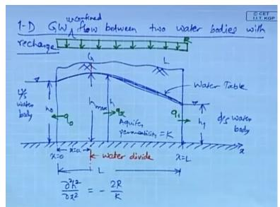
So here as you can see from the from the figure due to this concept or uniform rate of recharge over in the vertically downward direction the water shows the hump somewhere in the middle where the this H values maximum = H Max. And so from there he water table dips slightly towards the upstream water body to the left and then more towards the water body to the right of this and this this section is known as the water divide.
