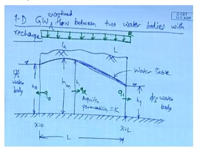
So let us say 1D ground water flow between two water bodies one day ground water unconfined flow with recharge. So let us consider unconfined ground water flow and let this be the upstream
