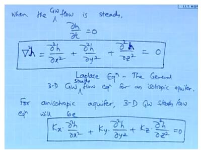
So when the flow ground water flow is steady in that case this DH / DT = 0 so therefore D square H / DX square + D square H / DY square + D square Z D I am sorry D square H / DZ square = 0 and obviously this is del square of H. So del square H which is = D square H / DX square + D square H / DZ square + D square H / DZ square which is = 0.
