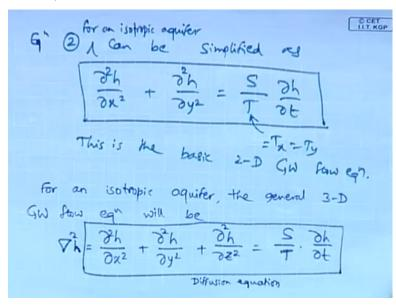
So we are continuing with the previous lecture so where in we went for we derived an expression for the two dimensional general ground water flow equation for an isotropic aquifer. So which is of the form D square H / DX square + D square H / Y square = S / T into DH / DT where here H represent the H, X and Y represents the flow direction S is the storativity T is transmissitivity and since it is a isotropic aquifer the transmissivity in both the directions DX and DY are same = T.
