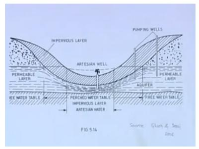
So this is a the you must have heard of the artesian well and here so in this artesian well it is basically it was developed initially somewhere in France in a place called Artois and in this cases this place is basically a pressurized well. So here have that is free water table is somewhere here and then in this region where the ground surface is below the free water table.
