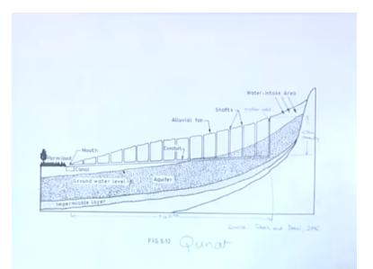
So this is a typical connate as you can see here in this this is a horizontal so this is essentially is the connate and the this the deepest well is known as mother well and this is the water intake area so basically this is a hilly area or a mountainous area where there is a significant amount of rainfall and this mother well as a depth of around 50 meters or less than that and there have been examples of mother well which are even as deeps as 100 meters.
