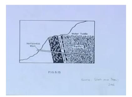
And here let me also show you an example of horizontal well as you can see here is an aquifer with water table here and that is the there is a sloping slide and this aquifer is bounded by impair case barrier and then say some rock formation here so through this there is a this horizontal well and of course the depending upon the water table. So this we can ground water can be harnessed through this horizontal valley well.
