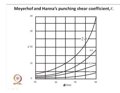
So; that means, here this Ks value will be required calculating the ultimate load carrying capacity of this layer soil. So, that case term is there as in the as you have seen then in this final expression. So, there we will be use the case. So, that is for the, if this phi 1. So, top layer if it is stronger sand because it is we are getting the case for the phi 1.
