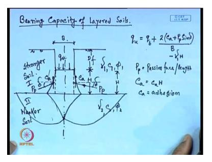
Now, suppose if we go for the bearing capacity of a layered soil system. Now, I will discuss the bearing capacity of layered soil. Now, the the derivation or the expression which is available for this to calculate the bearing capacity of the soil, which is basically for the homogeneous soil. Now, if the soil is in this form that this is the ground surface.
