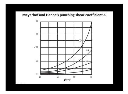
Now, if we go for this chart that this is the chart which is presented by Meyerhof and Hanna's 1978 is also the source is this book. Now, here this is as I have mentioned that this punching shear coefficient K s is function of q 2 by q 1 and phi 1. So, punching shear coefficient in the function of q 2 by q 1 and phi 1.
