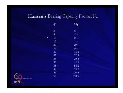
But for this n gamma factor Hansen's has recommended one table, that is to determine this corresponding to the phi value, then we can determine this n gamma factors for different phi value. This is varies from 0 degree to 50 degrees, these are the values of N q. So, by using the Meyerhof's table for Hansen's recommendation we can determine the N c and N q bearing capacity factor and by using this table we can determine the N gamma bearing capacity factor.
