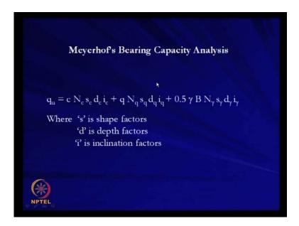
Now, the next one that we will discuss about the Meyerhof's bearing capacity analysis. Now, in this Terzaghi's bearing capacity analysis that it is assumed that this failure
