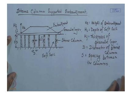
So, first if I go to that stone column supported embankment, so that thing that part, say, assume this is the embankment. Then below that we use a sand pad or granular layer; then this is the existing soil which is improved by stone columns. So, this was the problem; this is the hard stratum and this portion is improved by stone column or granular pile. So, these are equals; these are the diameter of the stone column and this is the spacing between the stone column and this is embankment.
