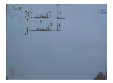
So, now if we produce this P 0 M 0 based on this two calculation, then we will get the condition or we get this case three or case c that this is infinite beam that is q and we apply a concentrated load and then at point A we are applying P 0 and M 0. So, that is equivalent to a fixed end beam a semi-infinite beam and this is q and this one is, this is A point and this is P 1. So, that means this is the third case where we will get this condition.
